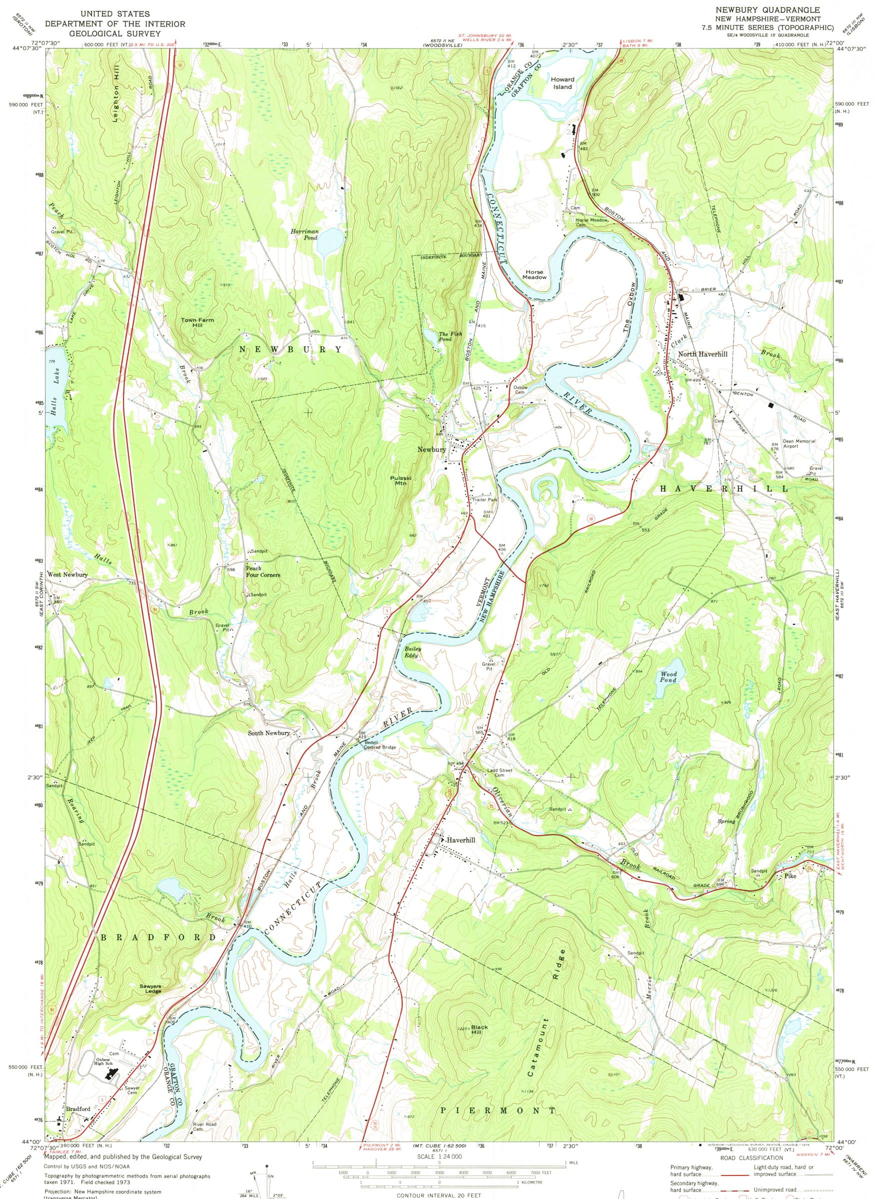
Projection: New Hampshire coordinate system (transverse Mercator) 10,000-foot grid ticks based on New Hampshire and Vermont coordinate systems 1000-metre Universal Transverse Mercator grid ticks, zone 18, shown in blue. 1927 North American datum Fine red dashed lines indicate selected fence and field lines where generally visible on aerial photographs. This information is unchecked
