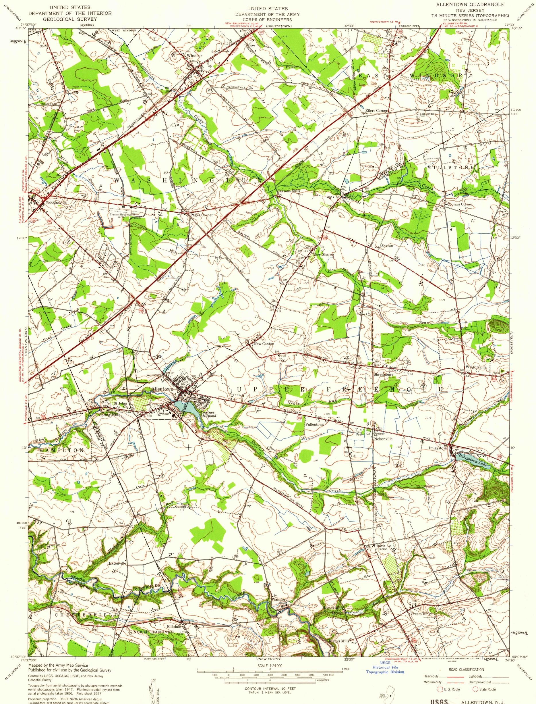
Aerial photographs taken 1947. Planimetric detail revised from aerial photographs taken 1956. Field check 1957 Polyconic projection. 1927 North American datum 10,000-foot grid based on New Jersey coordinate system 1000-meter Universal Transverse Mercator grid ticks, zone 18, shown in blue
