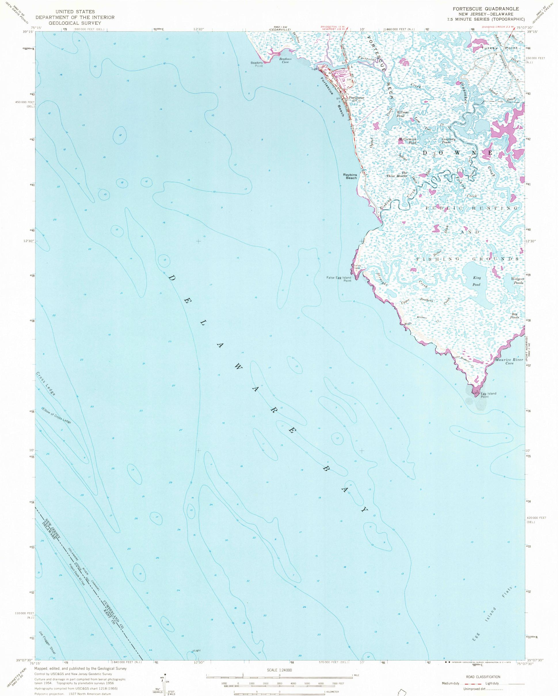
Polyconic projection. 1927 North American datum 10,000-foot grids based on New Jersey and Delaware coordinate systems. 1000-meter Universal Transverse Mercator grid ticks, zone 18, shown in blue
