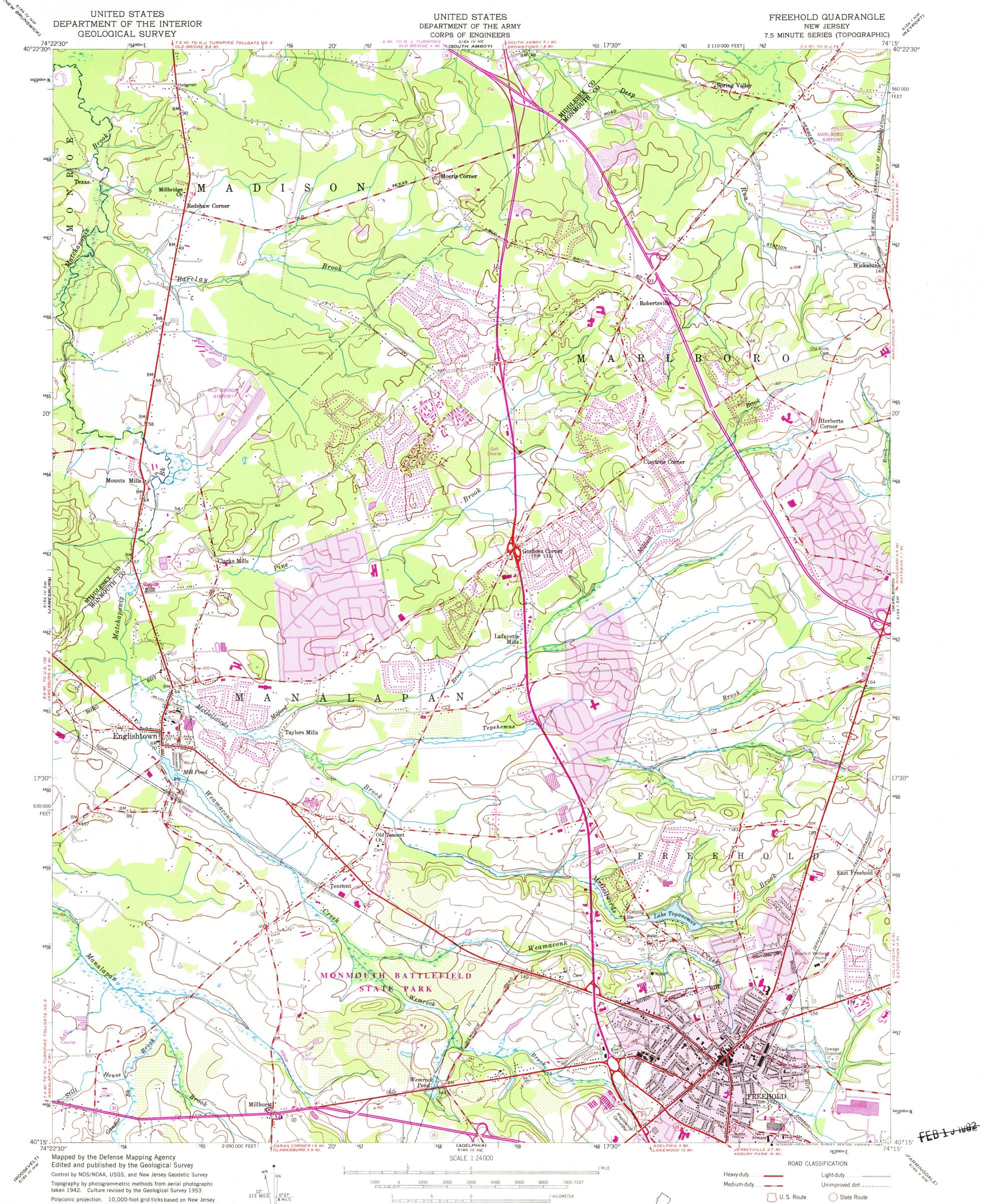
coordinate system. 1000-meter Universal Transverse Mercator grid ticks, zone 18, shown in blue. 1927 North American Datum. To place on the predicted North American Datum 1983 move the projection UTM GRID AND 1981 MAGNETIC NORTH DECLINATION AT CENTER OF SHEET lines 6 meters south and 34 meters west as shown by dashed corner ticks
