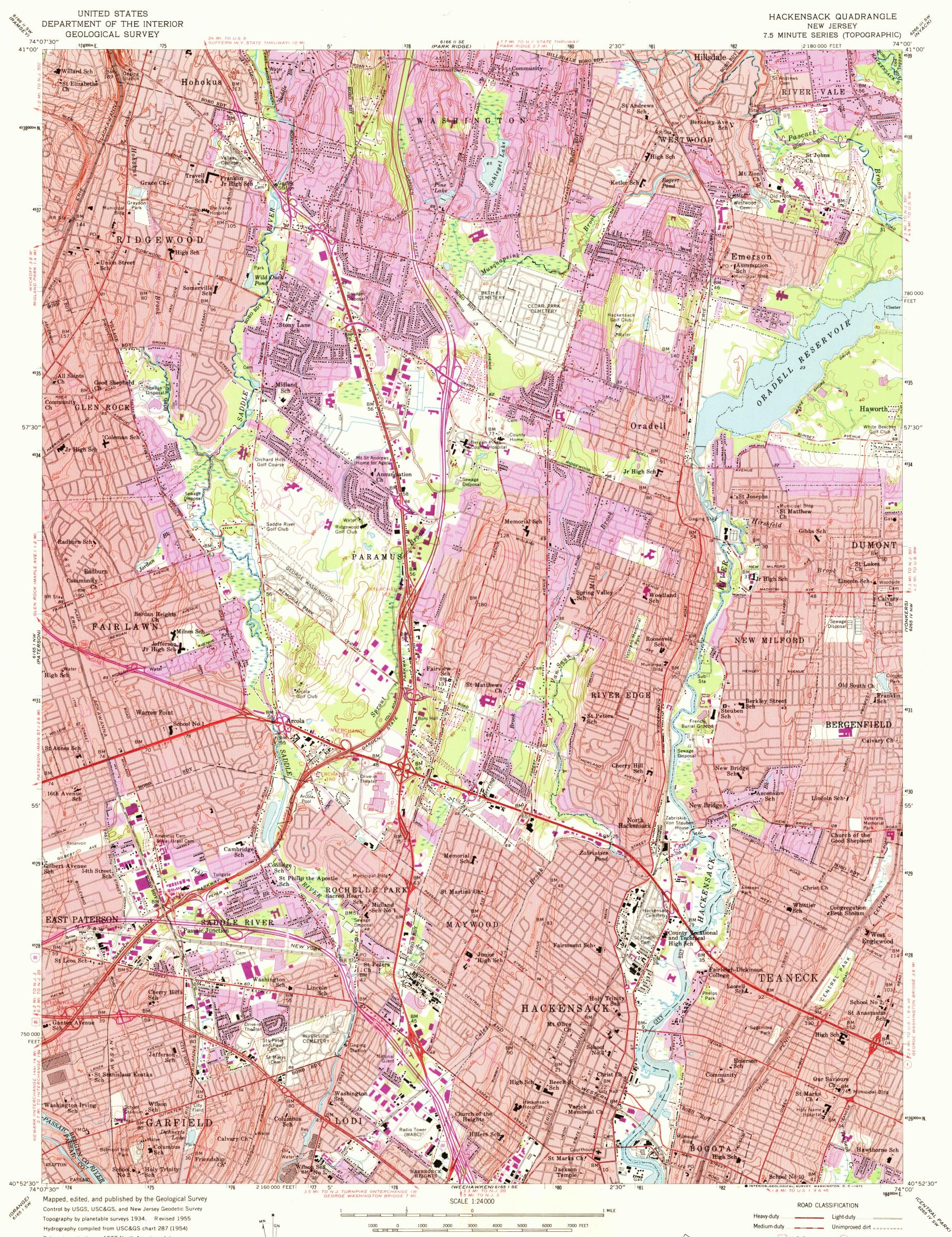
Polyconic projection. 1927 North American datum 10,000-foot grid based on New Jersey coordinate system 1000-meter Universal Transverse Mercator grid ticks, zone 18, shown in blue Red tint indicates areas in which only landmark buildings are shown
