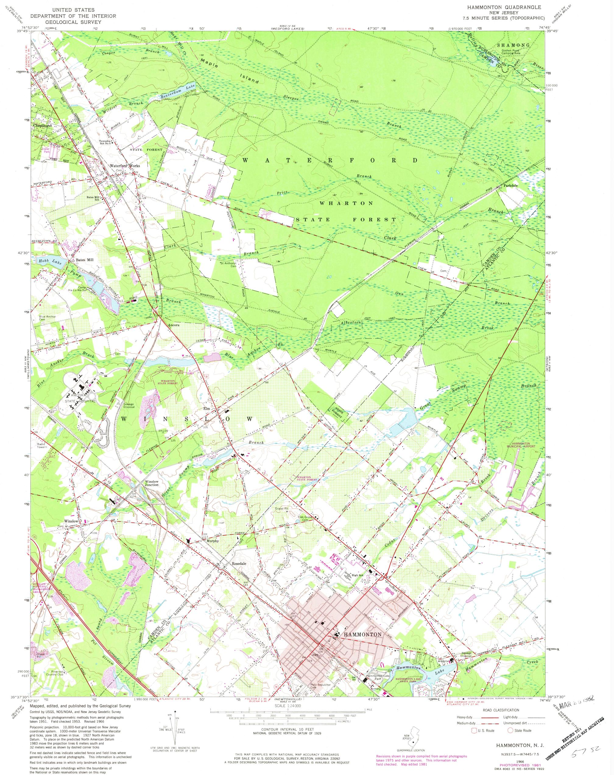
Polyconic projection. 10,000-foot grid based on New Jersey coordinate system. 1000-meter Universal Transverse Mercator grid ticks, zone 18, shown in blue. 1927 North American Datum. To place on the predicted North American Datum 1983 move the projection lines 6 meters south and 32 meters west as shown by dashed corner ticks Fine red dashed lines indicate selected fence and field lines where generally visible on aerial photographs. This information is unchecked
