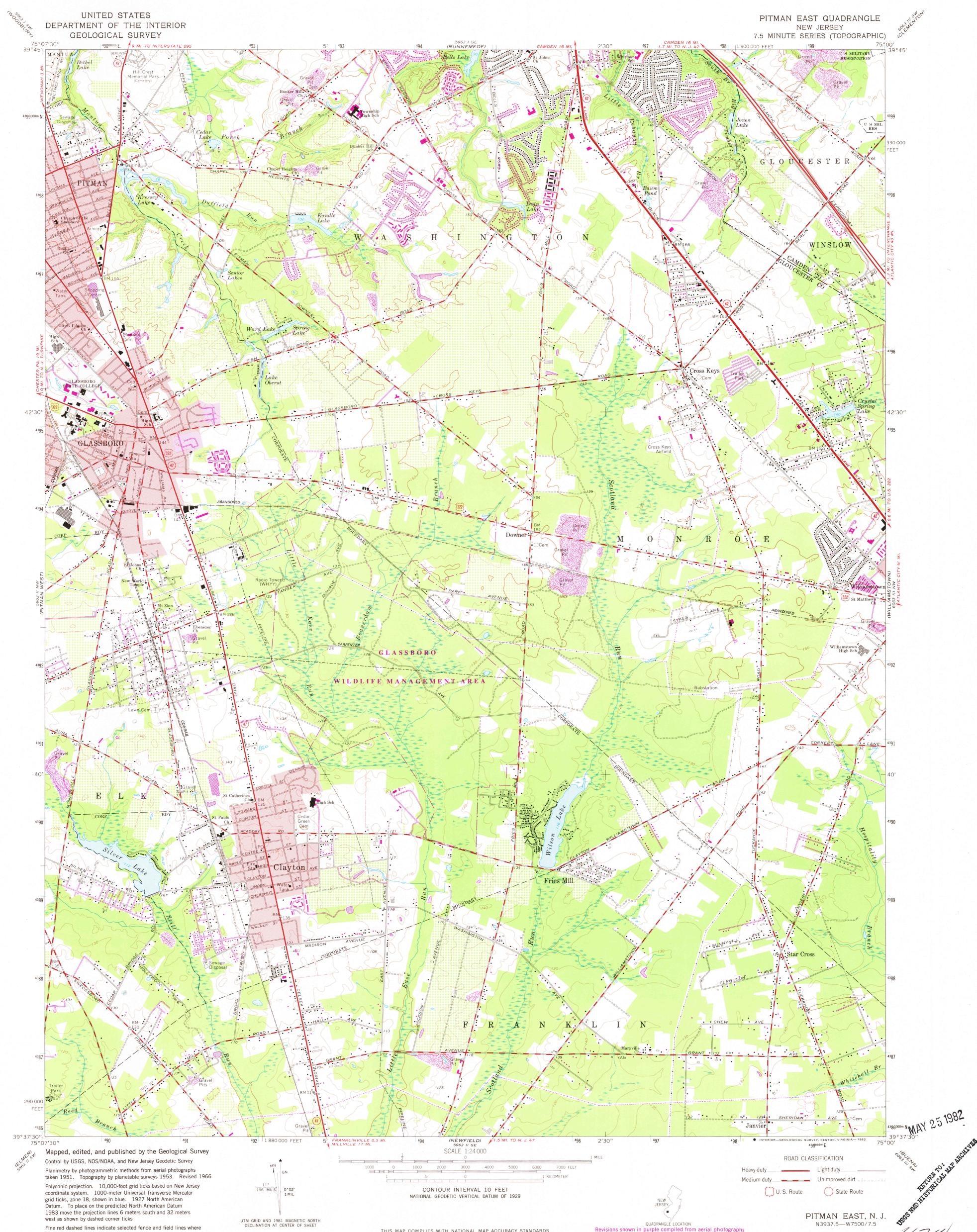
Polyconic projection. 10,000-foot grid ticks based on New Jersey coordinate system. 1000-meter Universal Transverse Mercator grid ticks, zone 18, shown in blue. 1927 North American Datum. To place on the predicted North American Datum 1983 move the projection lines 6 meters south and 32 meters west as shown by dashed corner ticks
