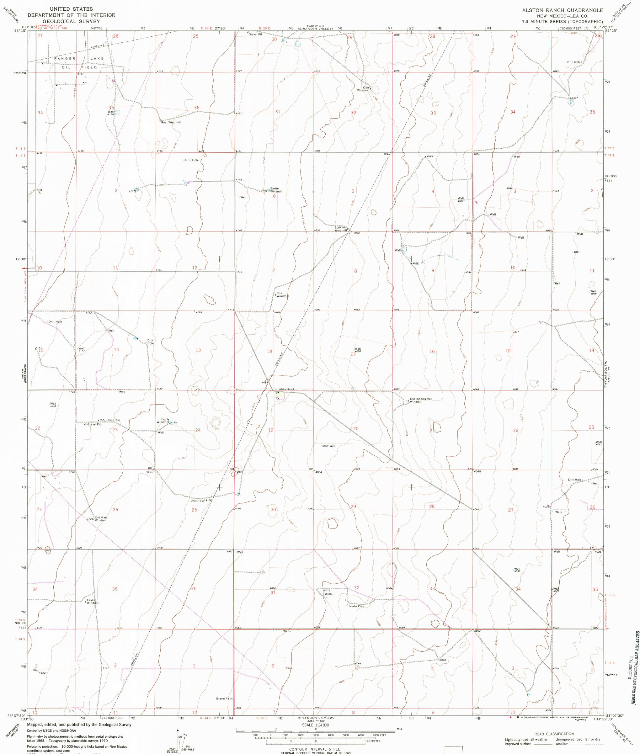
coordinate system, east zone 1000-meter Universal Transverse Mercator grid ticks, zone 13, shown in blue 1927 North American Datum To place on the predicted North American Datum 1983 move the projection lines 8 meters south and 46 meters east as shown by dashed corner ticks
