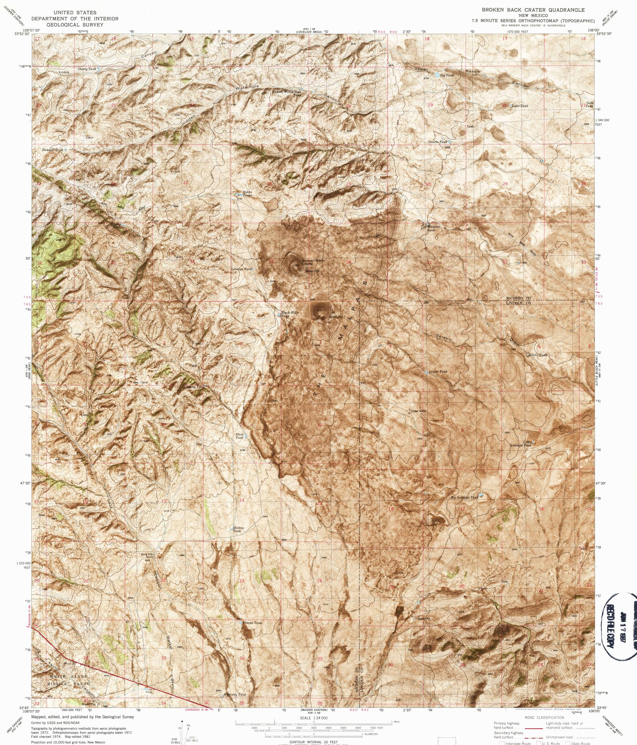
Projection and 10,000-foot grid ticks: New Mexico coordinate system, central zone (transverse Mercator) 1000-meter Universal Transverse Mercator grid, zone 13 1927 North American Datum To place on the predicted North American Datum 1983 move the projection lines 4 meters south and 51 meters east as shown by dashed corner ticks
