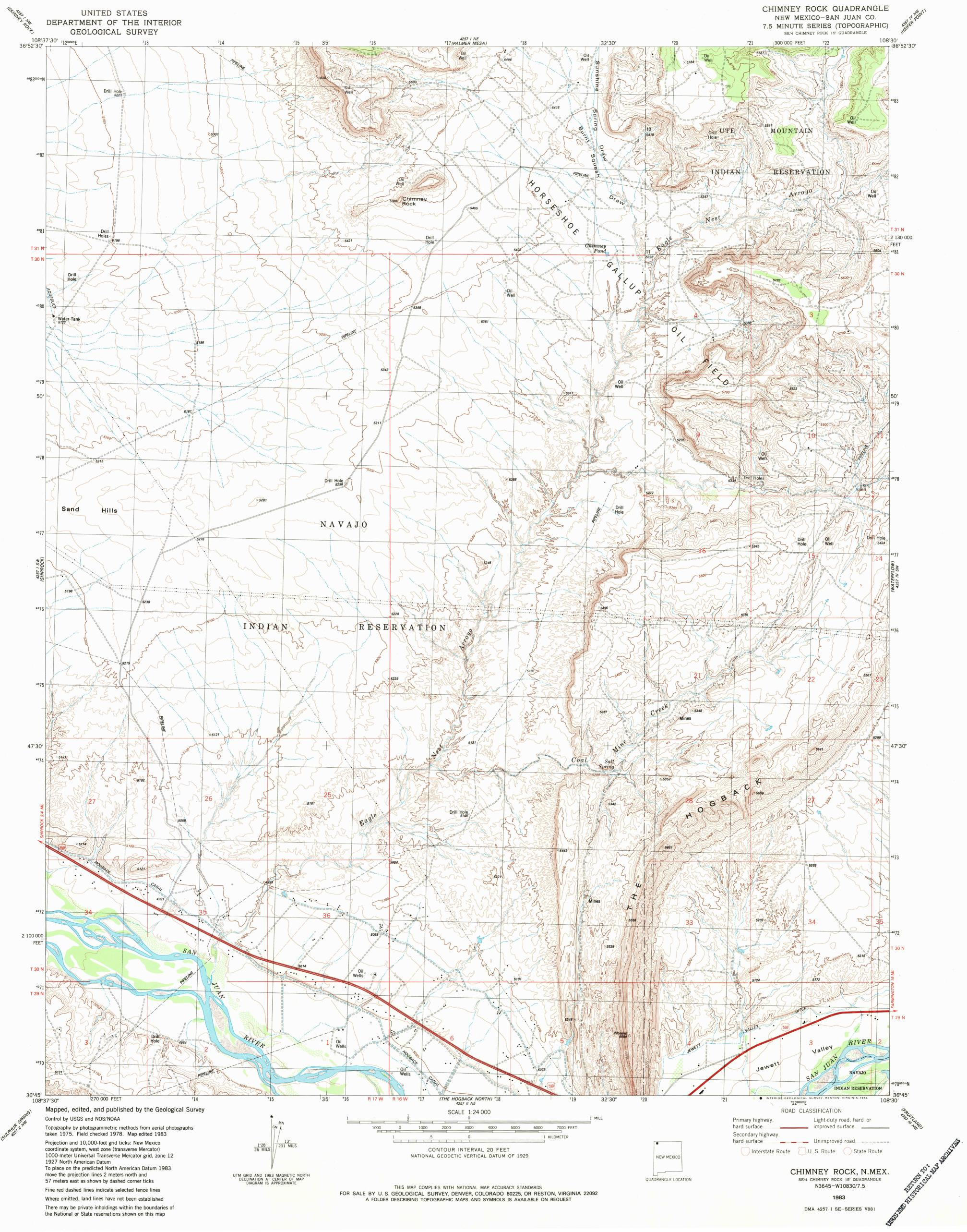
Projection and 10,000-foot grid ticks: New Mexico coordinate system, west zone (transverse Mercator) 1000-meter Universal Transverse Mercator grid, zone 12 1927 North American Datum To place on the predicted North American Datum 1983 move the projection lines 2 meters north and 57 meters east as shown by dashed corner ticks Fine red dashed lines indicate selected fence lines
