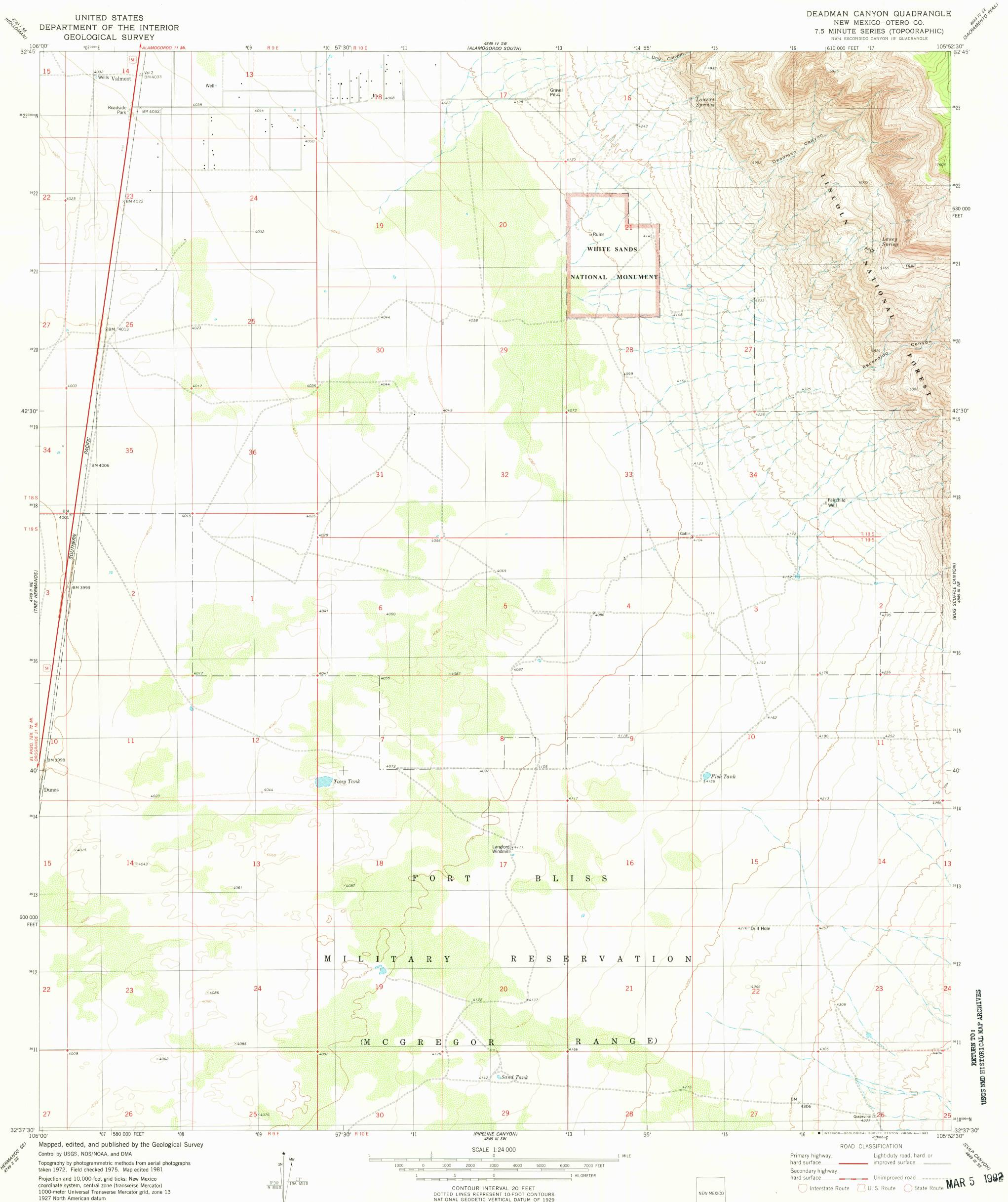
coordinate system, central zone (transverse Mercator) 1000-meter Universal Transverse Mercator grid, zone 13 1927 North American datum To place on the predicted North American Datum 1983 move the projection lines 6 meters south and 50 meters east as shown by dashed corner ticks
