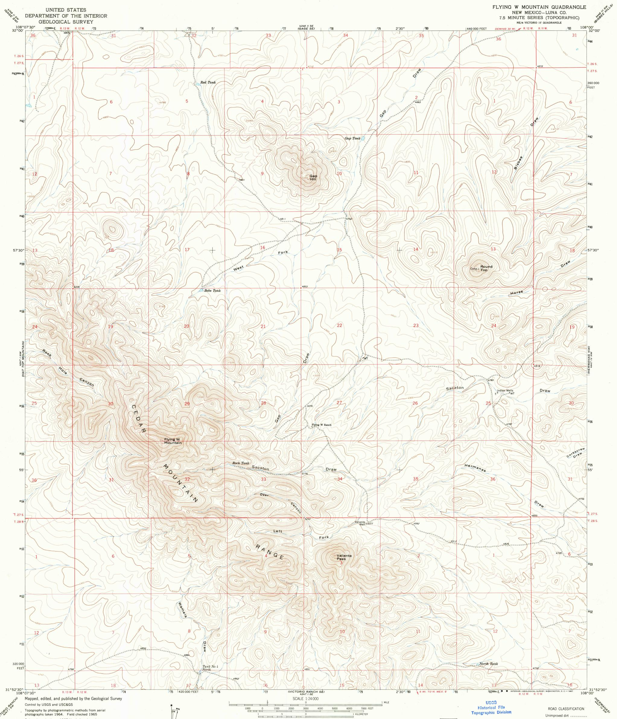
Polyconic projection. 1927 North American datum 10,000-foot grid based on New Mexico coordinate system, west zone 1000-meter Universal Transverse Mercator grid ticks, zone 12, shown in blue
