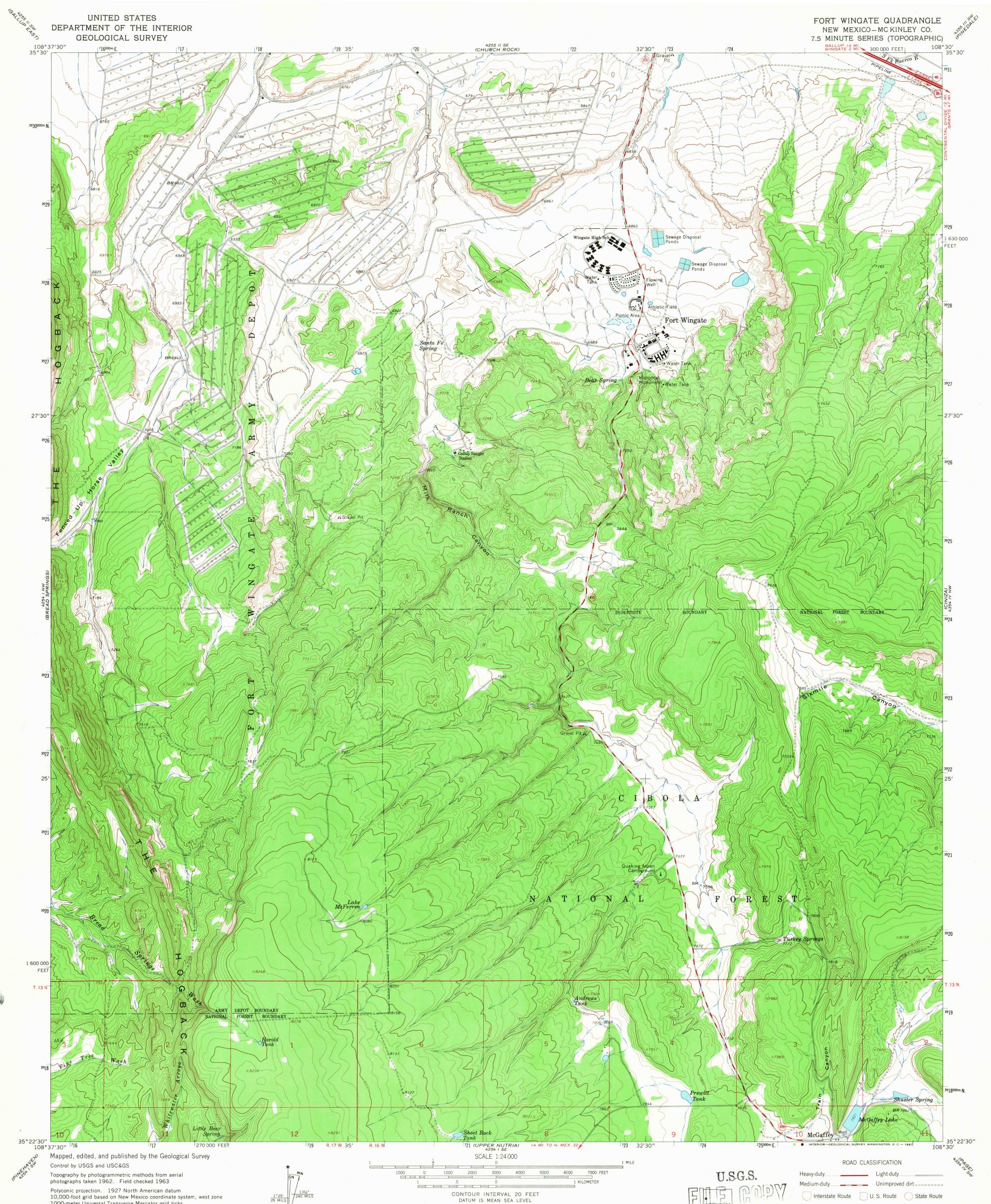
10,000-foot grid based on New Mexico coordinate system, west zone 1000-meter Universal Transverse Mercator grid ticks, zone 12, shown in blue
