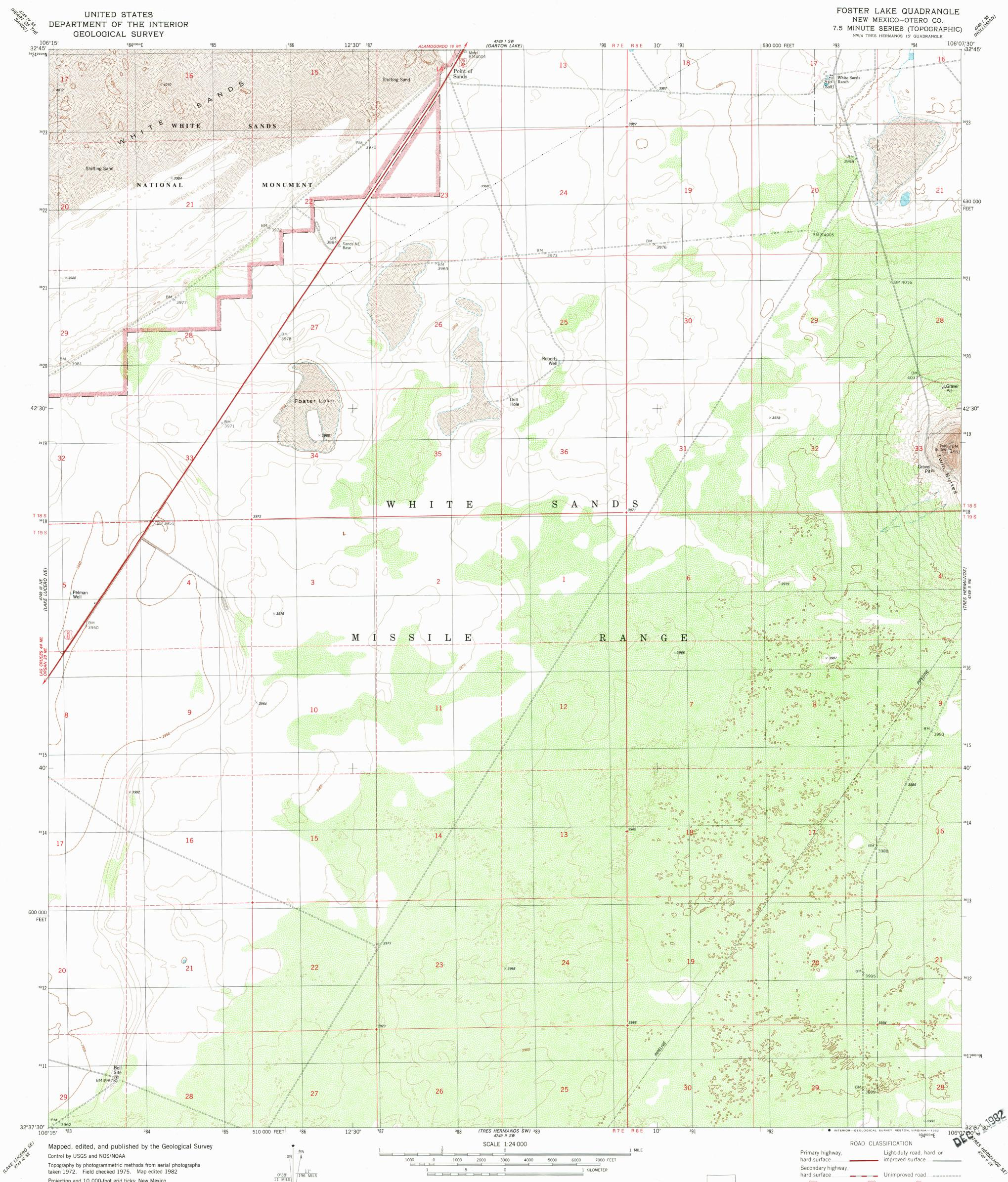
Projection and 10,000-foot grid ticks: New Mexico coordinate system, central zone (transverse Mercator) 1000-meter Universal Transverse Mercator grid, zone 13 1927 North American datum To place on the predicted North American Datum 1983 move the projection lines 6 meters south and 51 meters east as shown by dashed corner ticks Fine red dashed lines indicate selected fence lines There may be private inholdings within the boundaries of the National or State reservations shown on this map
