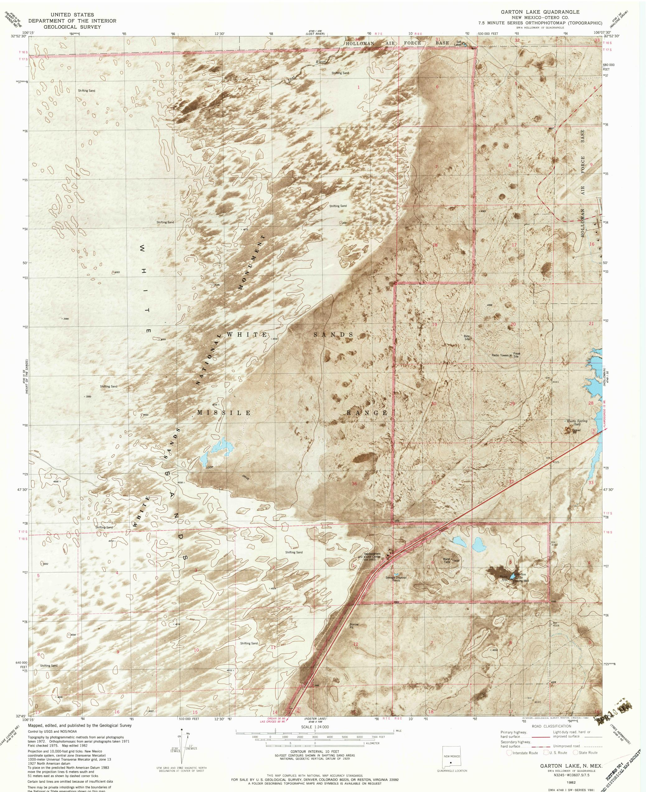
Projection and 10,000-foot grid ticks: New Mexico coordinate system, central zone (transverse Mercator) 1000-meter Universal Transverse Mercator grid, zone 13 1927 North American datum To place on the predicted North American Datum 1983 move the projection lines 6 meters south and 51 meters east as shown by dashed corner ticks Certain land lines are omitted because of insufficient data There may be private inholdings within the boundaries of the National or State reservations shown on this map
