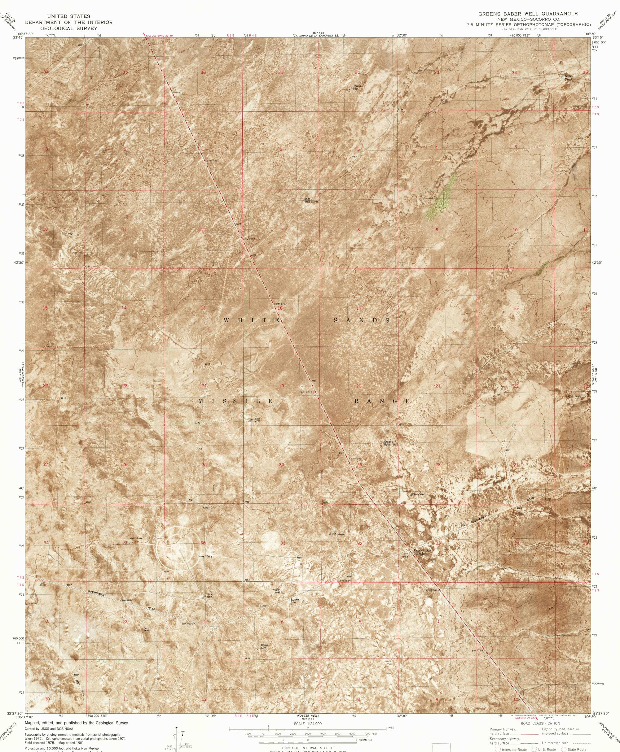
Projection and 10,000-foot grid ticks: New Mexico coordinate system, central zone (transverse Mercator) 1000-meter Universal Transverse Mercator grid, zone 13 1927 North American datum To place on the predicted North American Datum 1983 move the projection lines 4 meters south and 52 meters east as shown by dashed corner ticks
