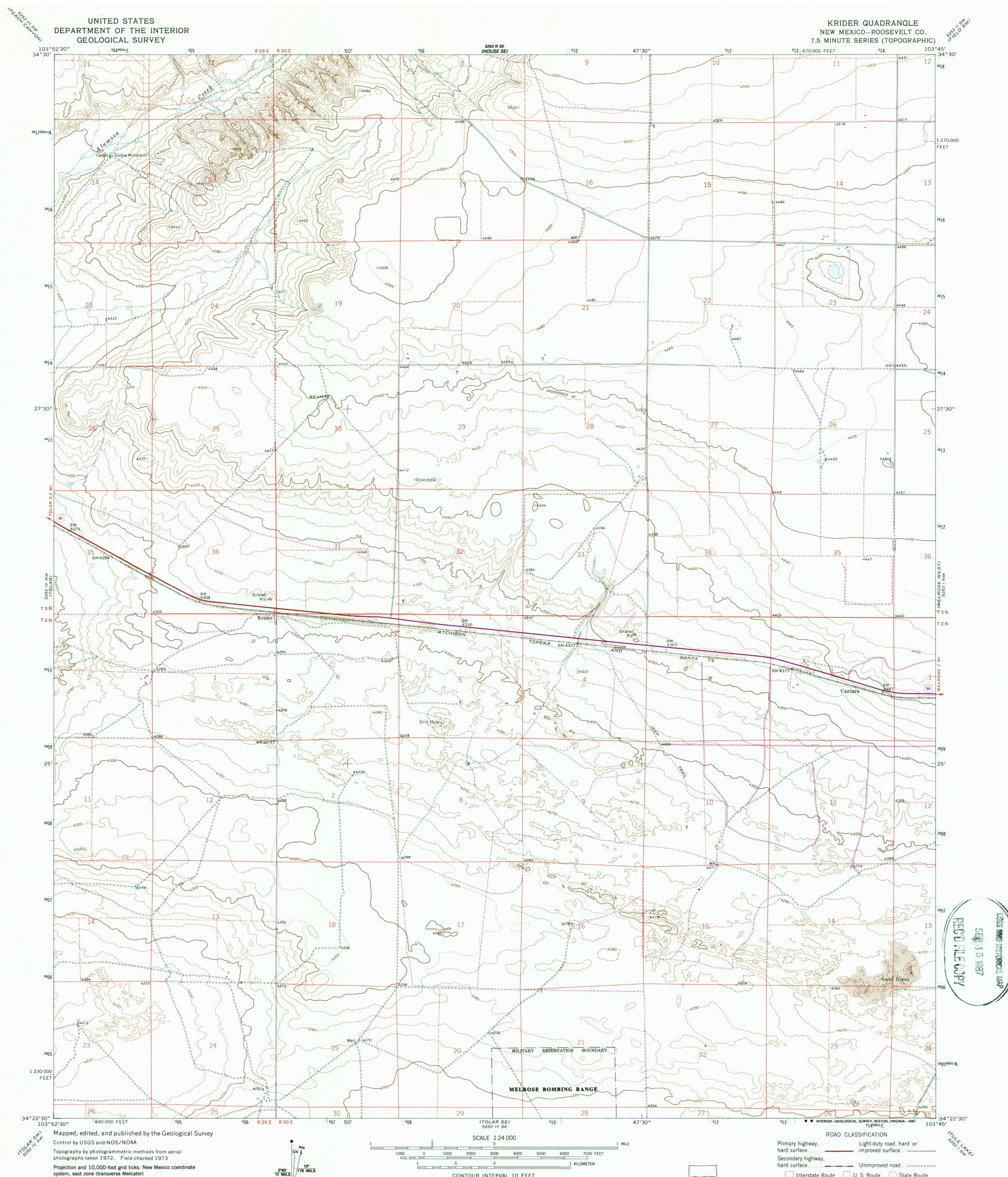
system, east zone (transverse Mercator) 1000-meter Universal Transverse Mercator grid ticks, zone 13, shown in blue. 1927 North American Datum To place on the predicted North American Datum 1983, move the projection lines 4 meters south and 46 meters east as shown by dashed corner ticks
