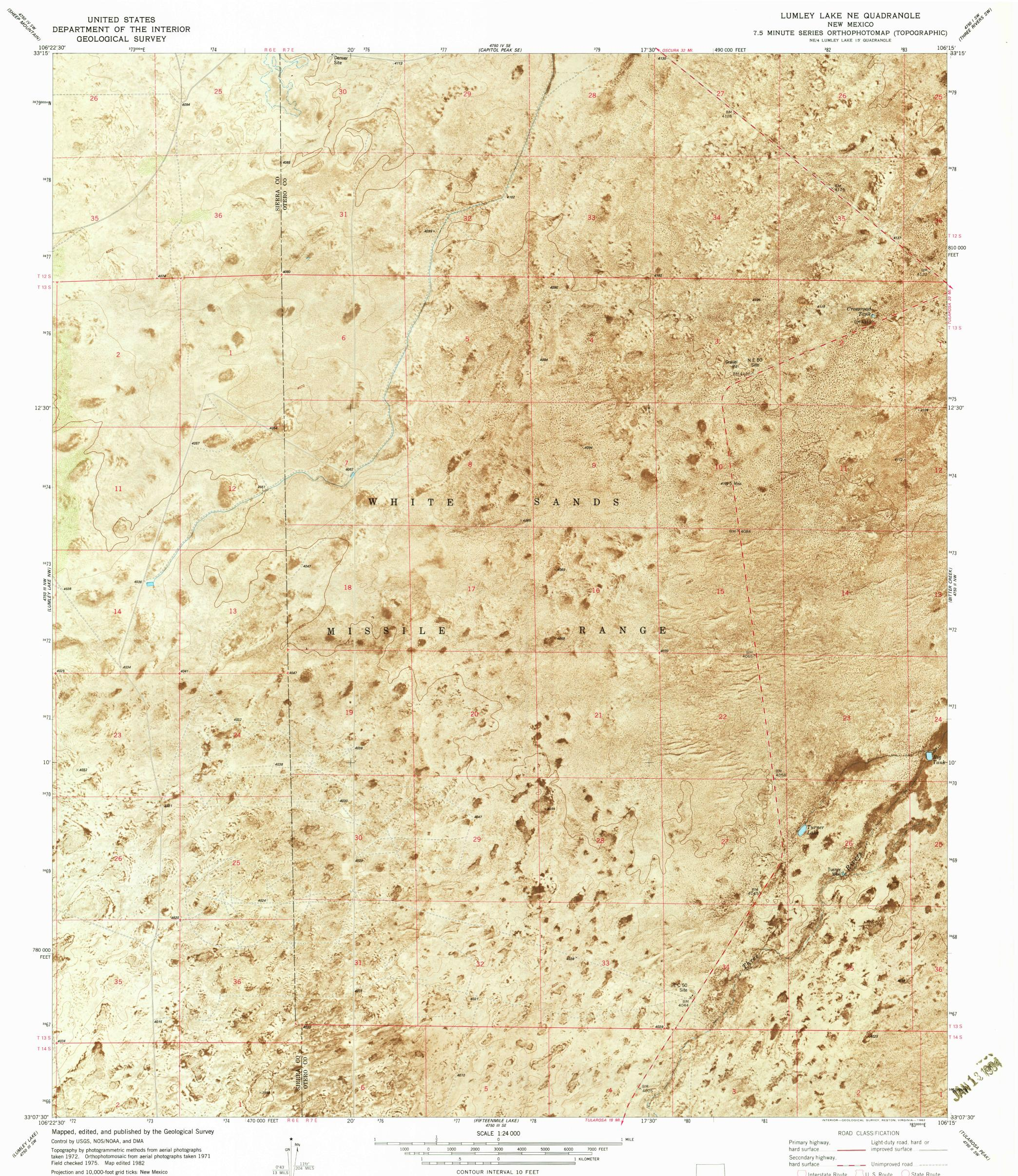
Projection and 10,000-foot grid ticks: New Mexico coordinate system, central zone (transverse Mercator) 1000-meter Universal Transverse Mercator grid, zone 13 1927 North American datum To place on the predicted North American Datum 1983 move the projection lines 5 meters south and 51 meters east as shown by dashed corner ticks There may be private inholdings within the boundaries of the National or State reservations shown on this map
