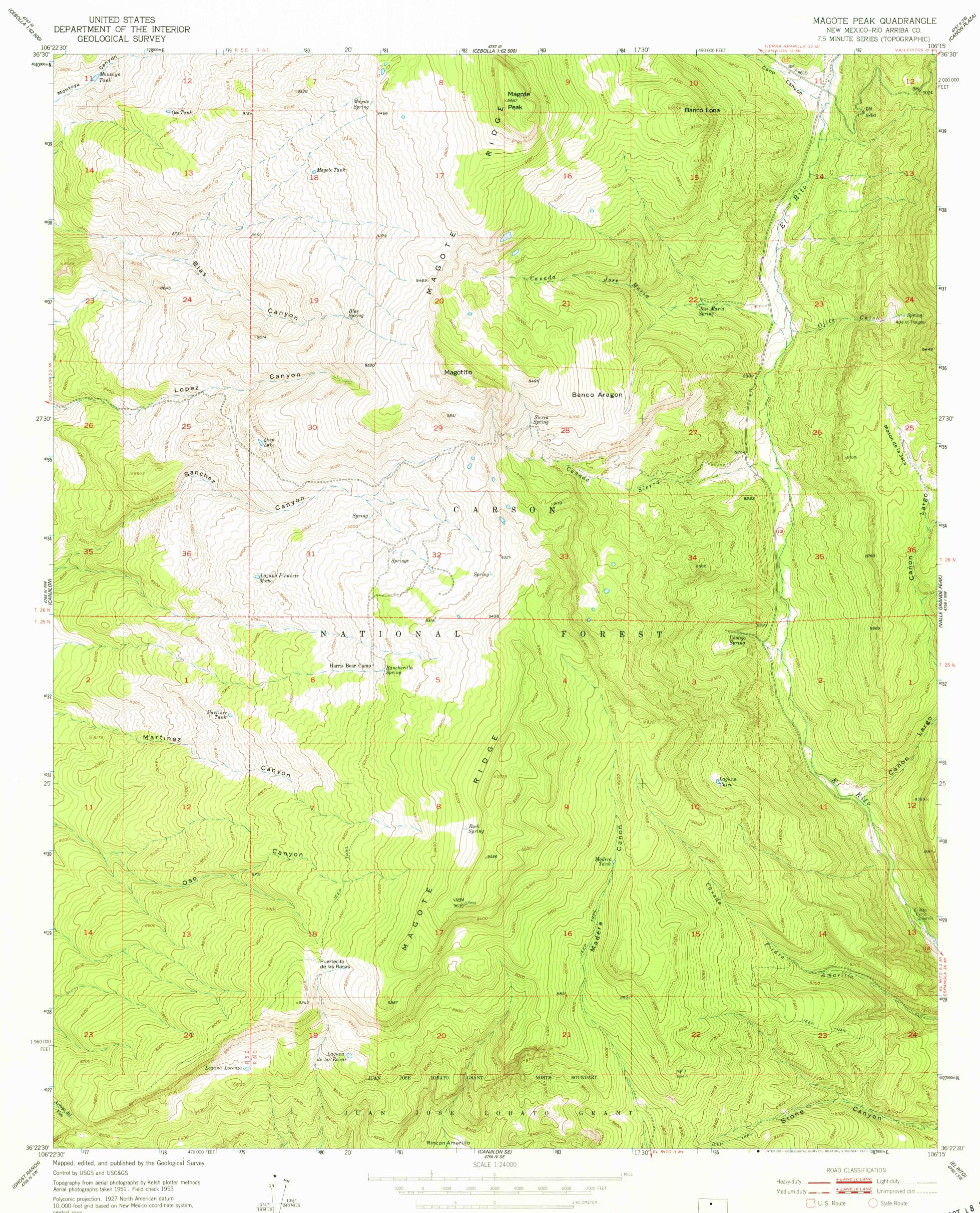
Polyconic projection. 1927 North American datum 10,000-foot grid based on New Mexico coordinate system, central zone Dashed land lines indicate approximate locations Unchecked elevations are shown in brown 1000-meter Universal Transverse Mercator grid ticks, zone 13, shown in blue
