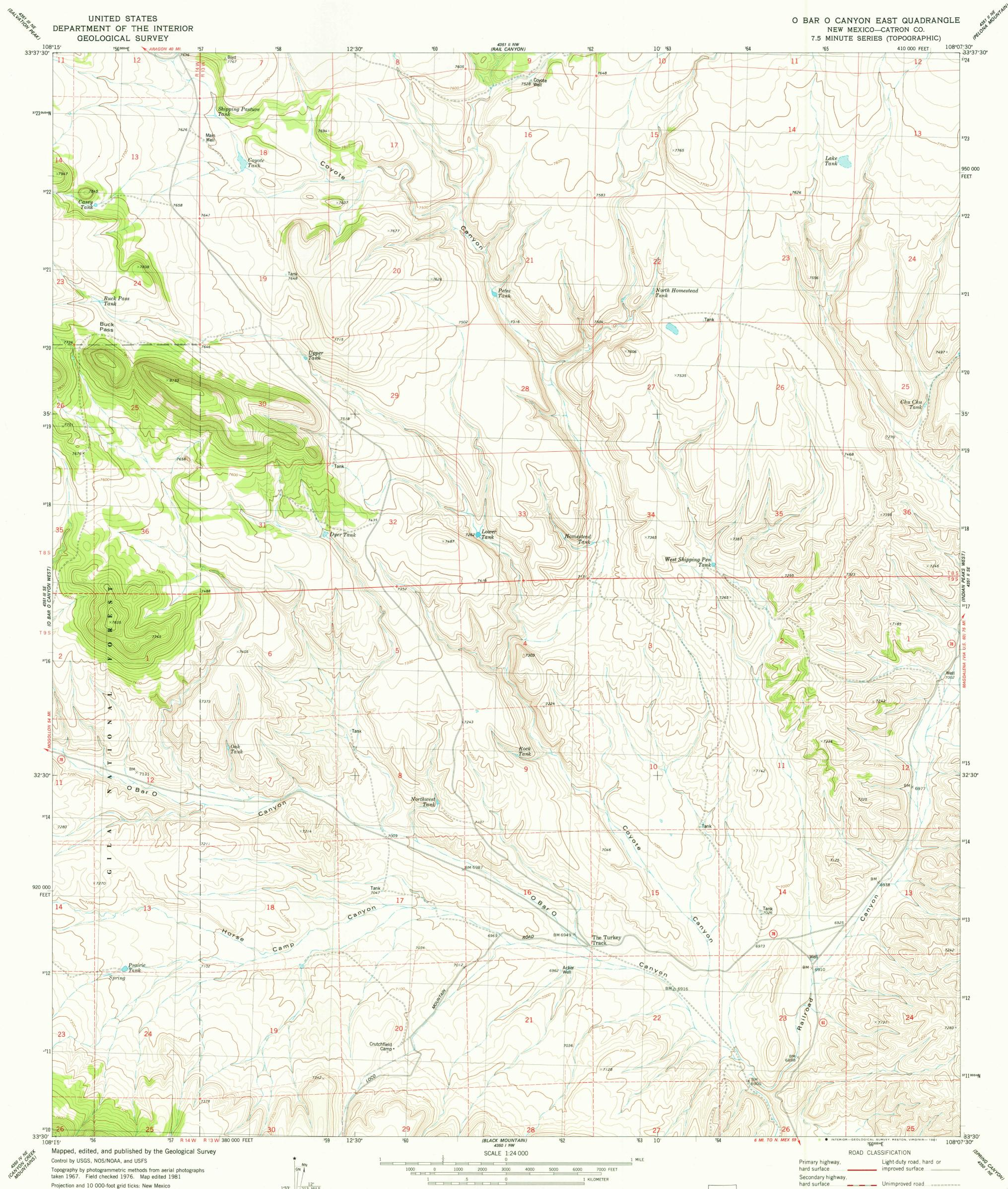
coordinate system, west zone (transverse Mercator) 1000-meter Universal Transverse Mercator grid, zone 12 1927 North American datum To place on the predicted North American Datum 1983 move the projection lines 4 meters south and 56 meters east as shown by dashed corner ticks Fine red dashed lines indicate selected fence lines
