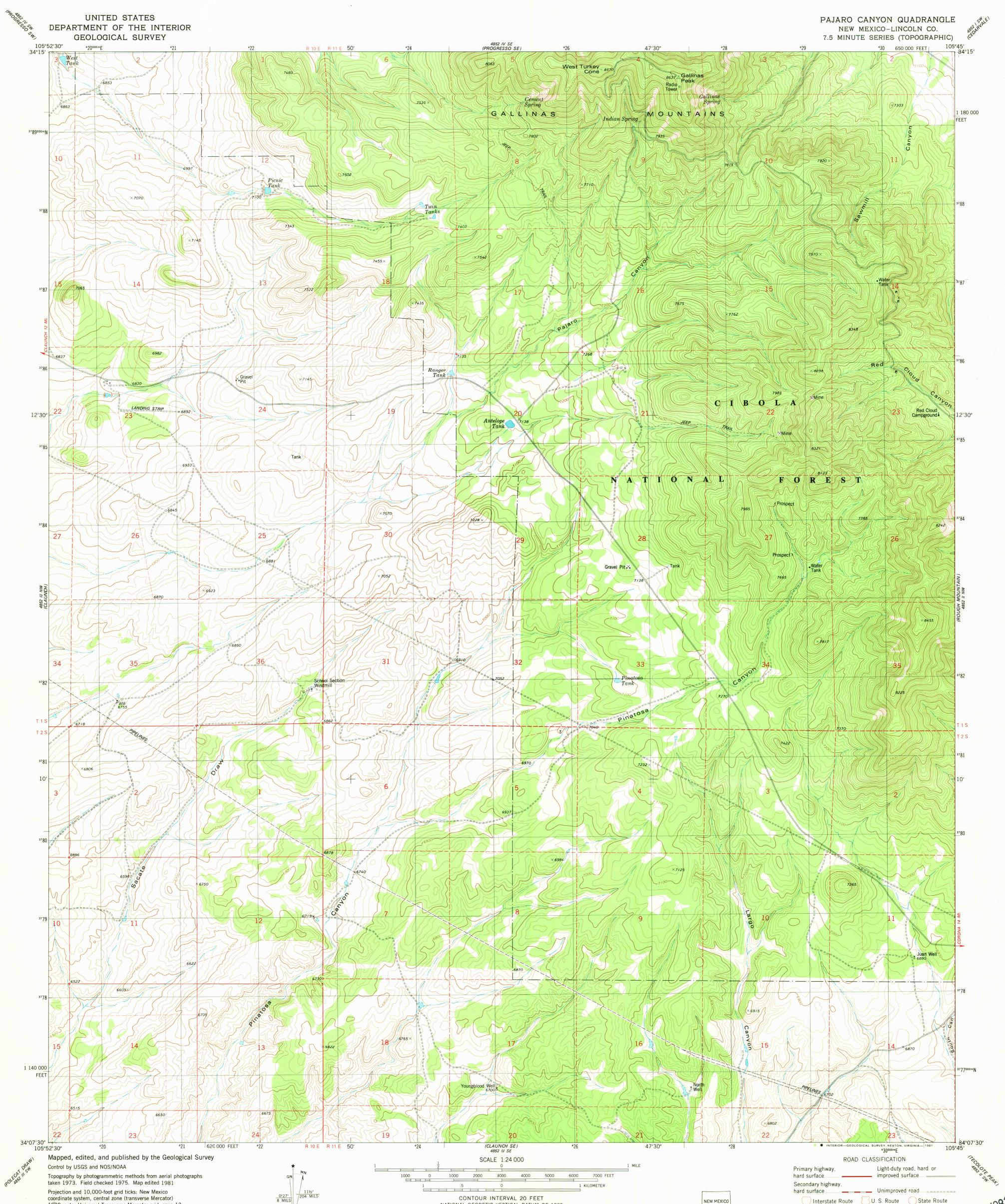
coordinate system, central zone (transverse Mercator) 1000-meter Universal Transverse Mercator grid, zone 13 1927 North American datum To place on the predicted North American Datum 1983 move the projection lines 4 meters south and 50 meters east as shown by dashed corner ticks
