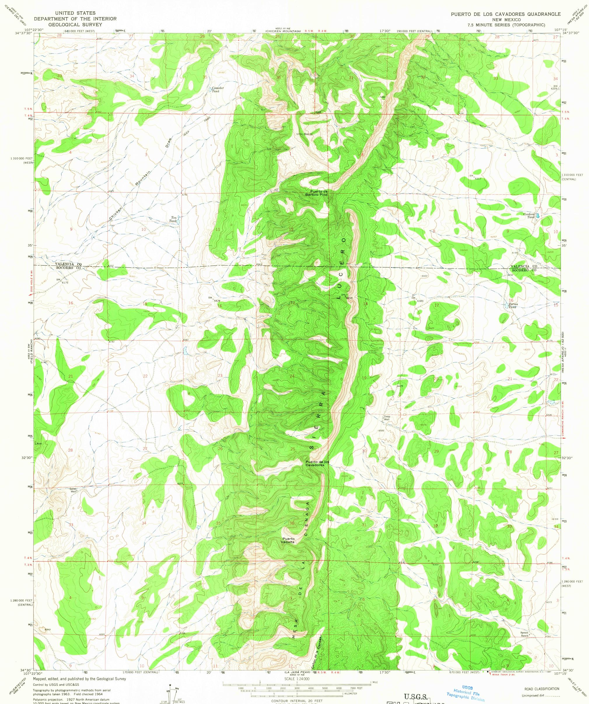
Polyconic projection. 1927 North American datum 10,000 foot grids based on New Mexico coordinate system, central and west zones 1000-meter Universal Transverse Mercator grid ticks, zone 13, shown in blue
