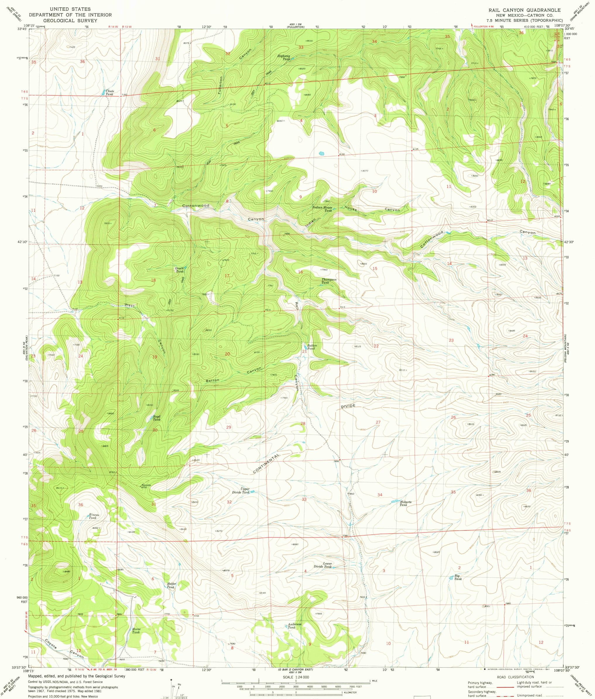
coordinate system, west zone (transverse Mercator) 1000-meter Universal Transverse Mercator grid, zone 12 1927 North American datum To place on the predicted North American Datum 1983 move the projection lines 4 meters south and 56 meters east as shown by dashed corner ticks
