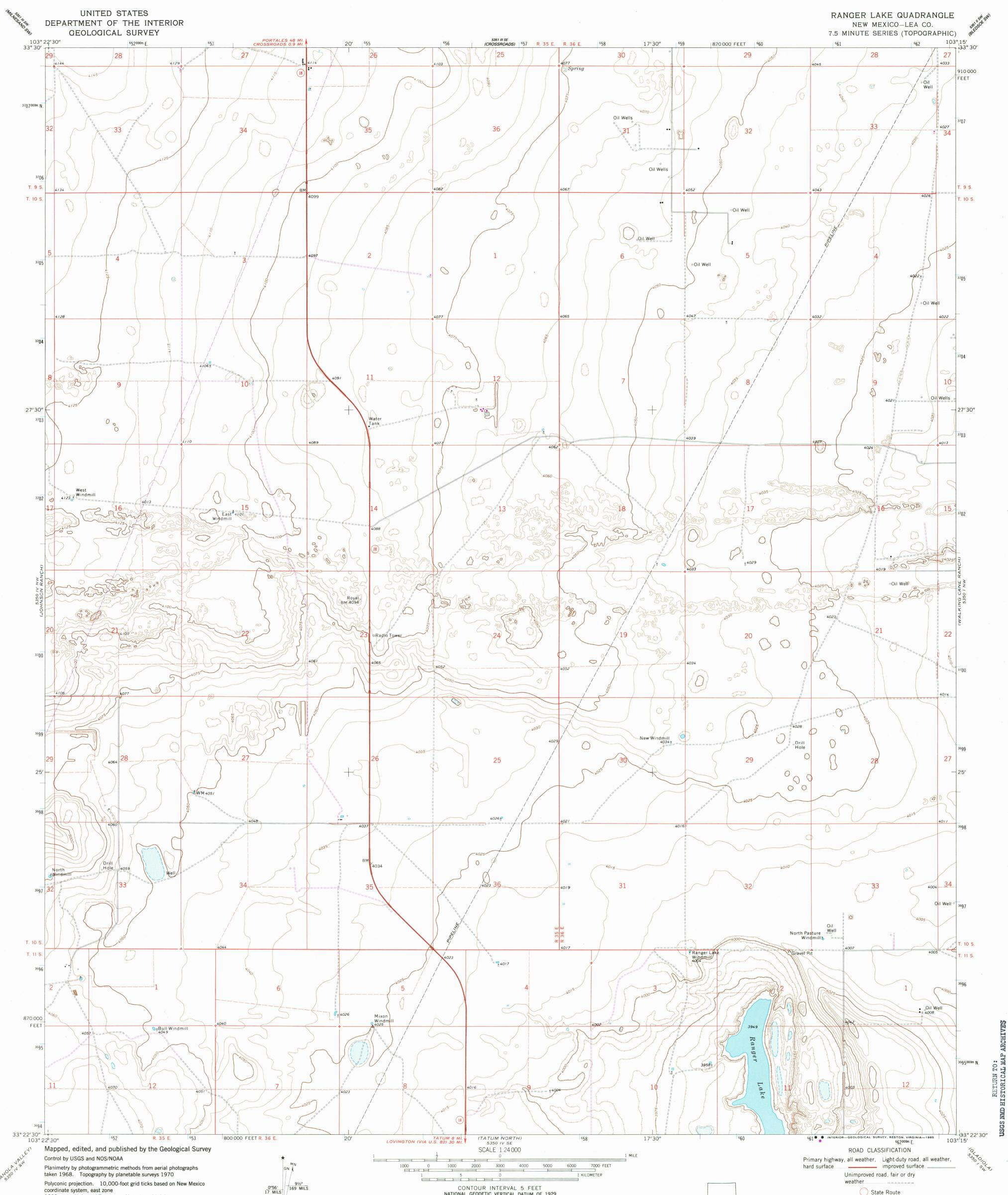
coordinate system, east zone 1000-meter Universal Transverse Mercator grid ticks, zone 13, shown in blue 1927 North American Datum To place on the predicted North American Datum 1983 move the projection lines 7 meters south and 45 meters east as shown by dashed corner ticks
