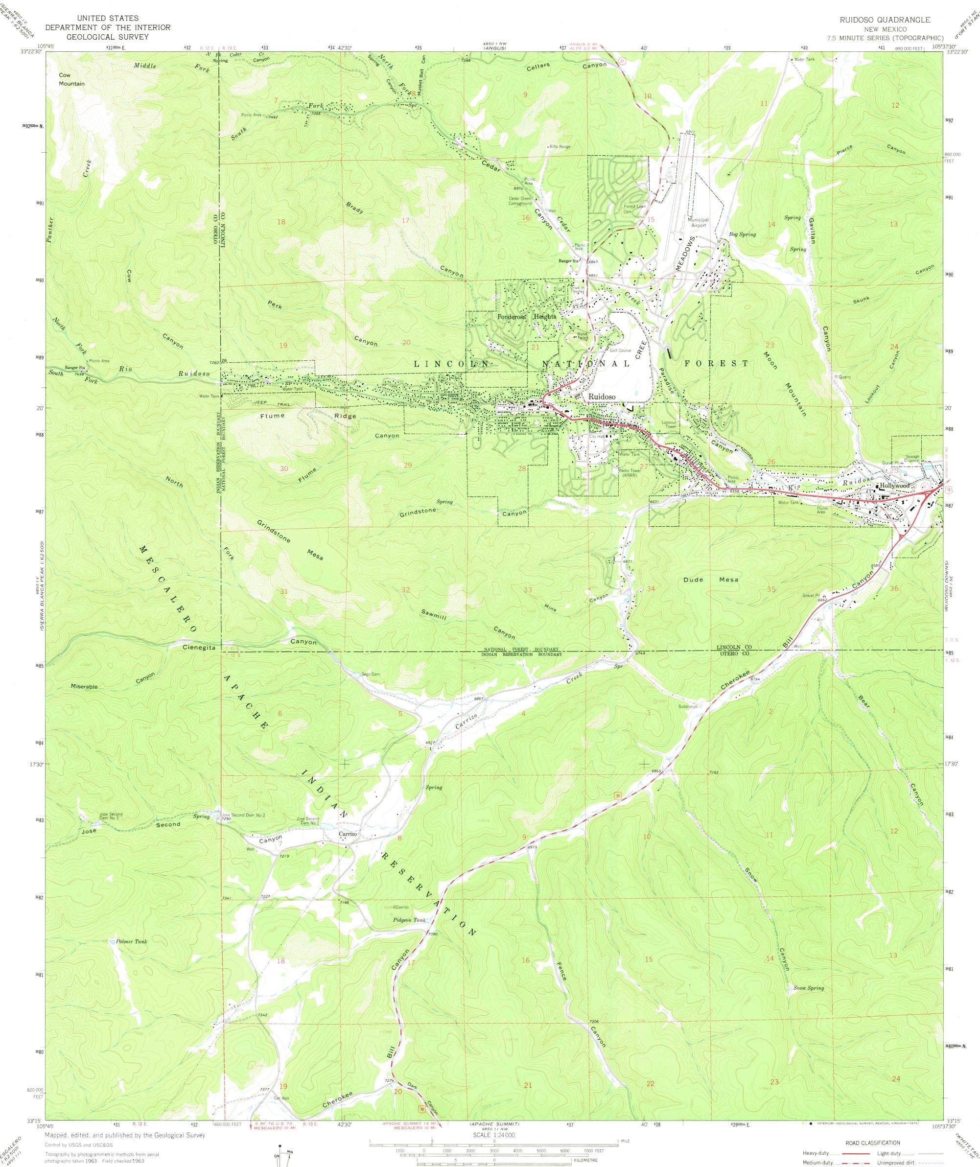
Polyconic projection. 1927 North American datum 10,000 foot grid based on New Mexico coordinate system, central zone 1000-metre Universal Transverse Mercator grid ticks, zone 13, shown in blue
