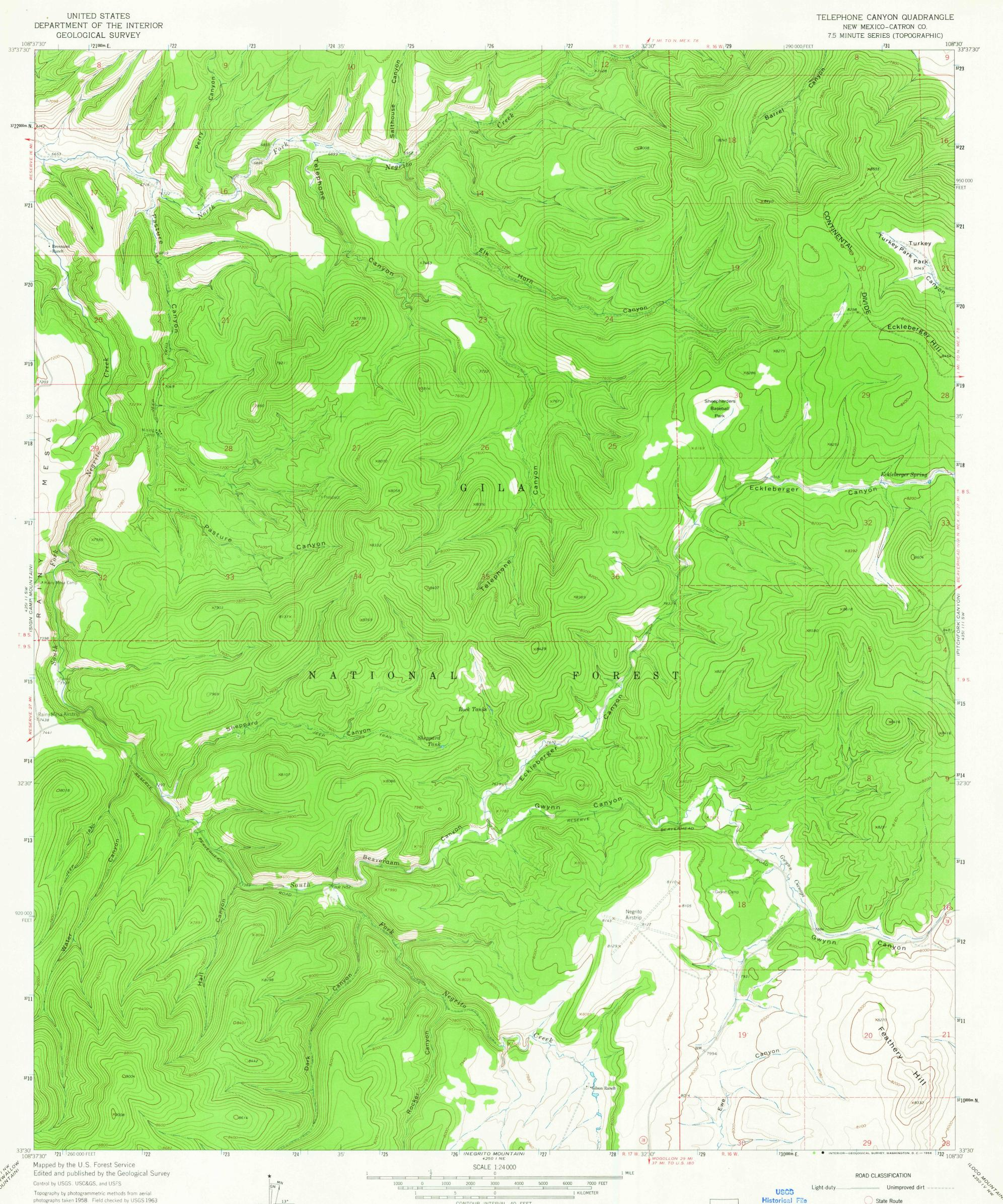
Polyconic projection. 1927 North American datum 10.000-foot grid based on New Mexico coordinate system, west zone 1000-meter Universal Transverse Mercator grid ticks, zone 12, shown in blue
