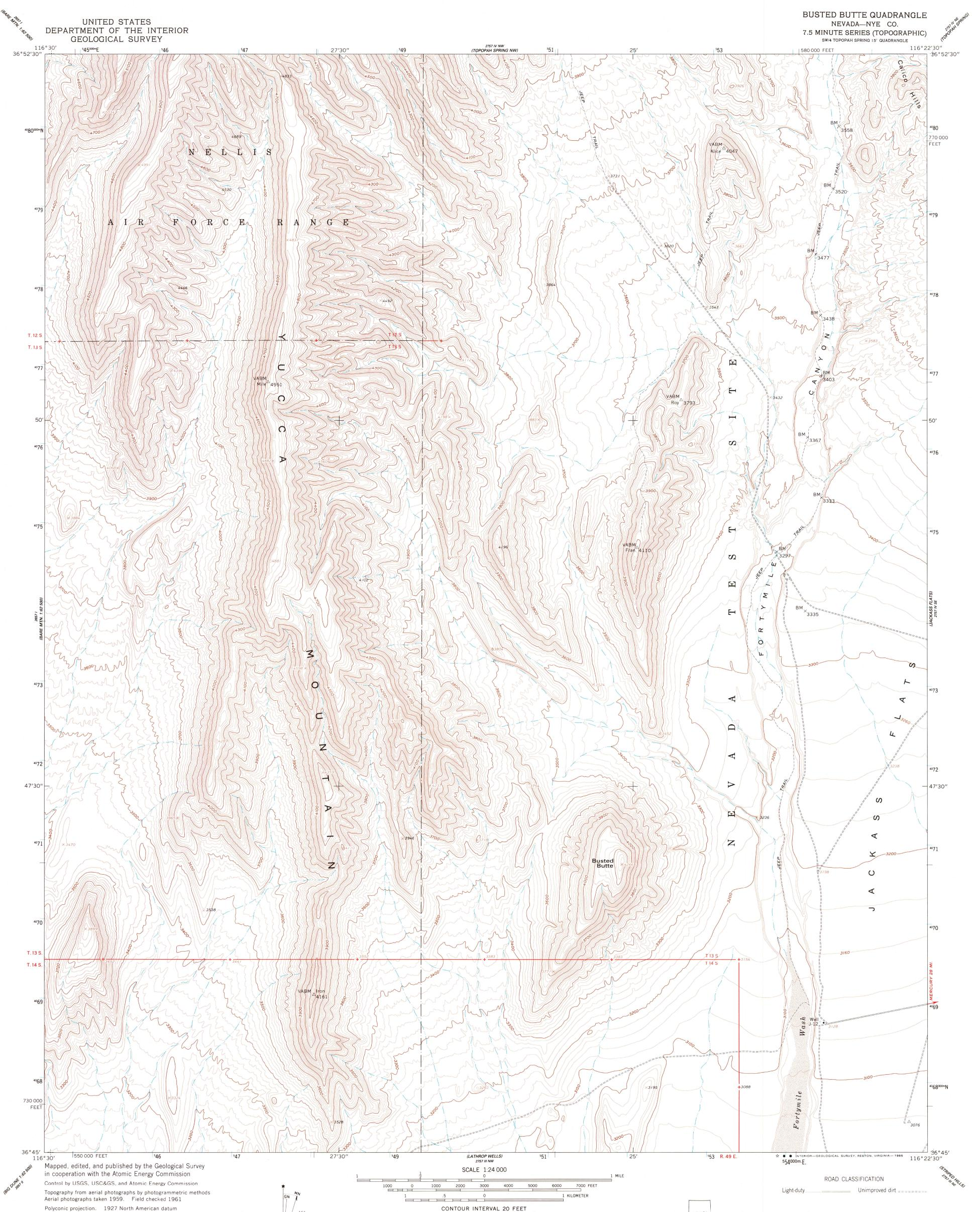
Polyconic projection. 1927 North American datum 10,000-foot grid based on Nevada coordinate system, central zone 1000-meter Universal Transverse Mercator grid ticks, zone 11, shown in blue To place on the predicted North American Datum 1983 move the projection lines 8 meters north and 78 meters east as shown by dashed corner ticks There may be private inholdings within the boundaries of the National or State reservations shown on this map
