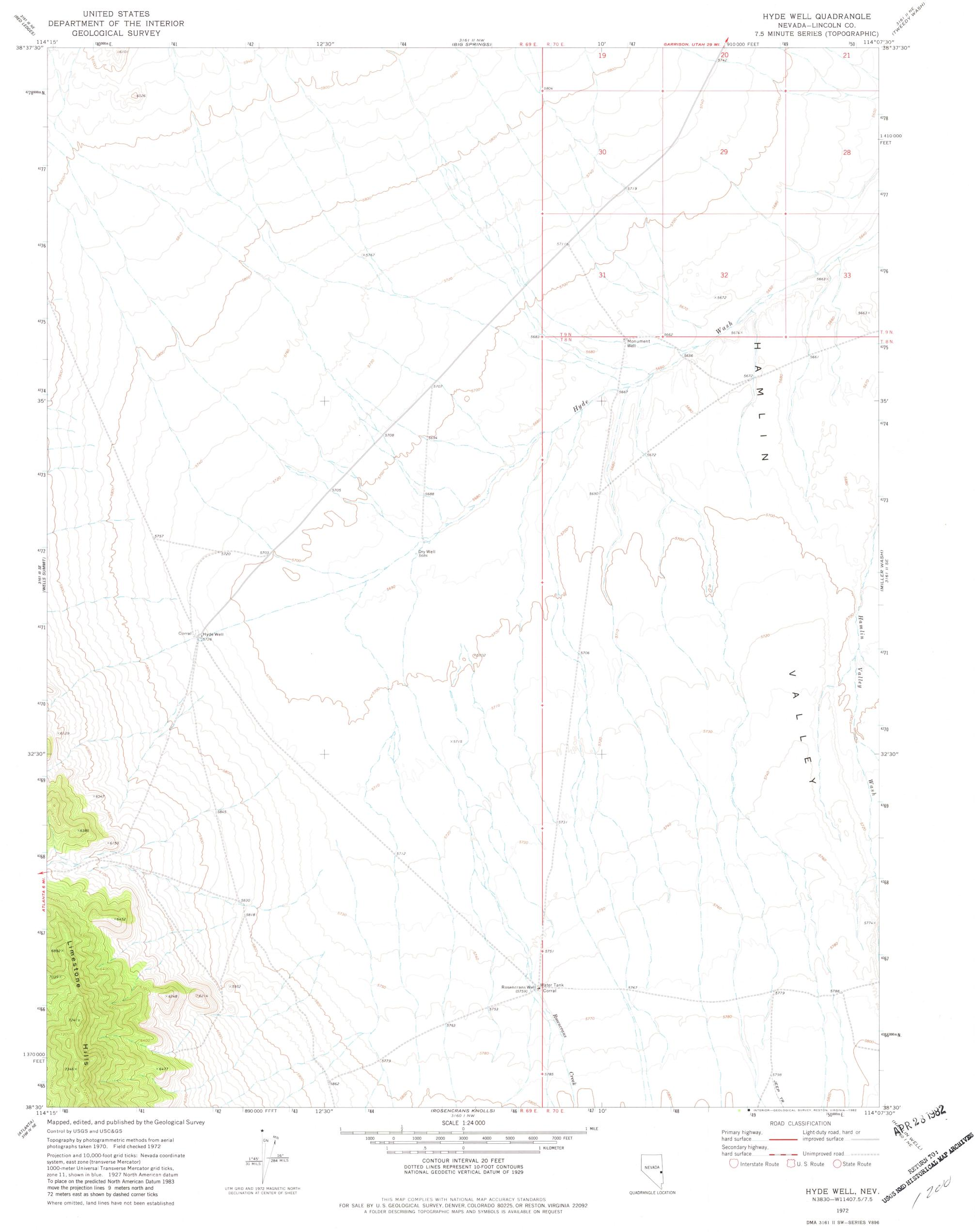
system, east zone (transverse Mercator) 1000-meter Universal Transverse Mercator grid ticks, zone 11, shown in blue. 1927 North American datum To place on the predicted North American Datum 1983 move the projection lines 9 meters north and 72 meters east as shown by dashed corner ticks
