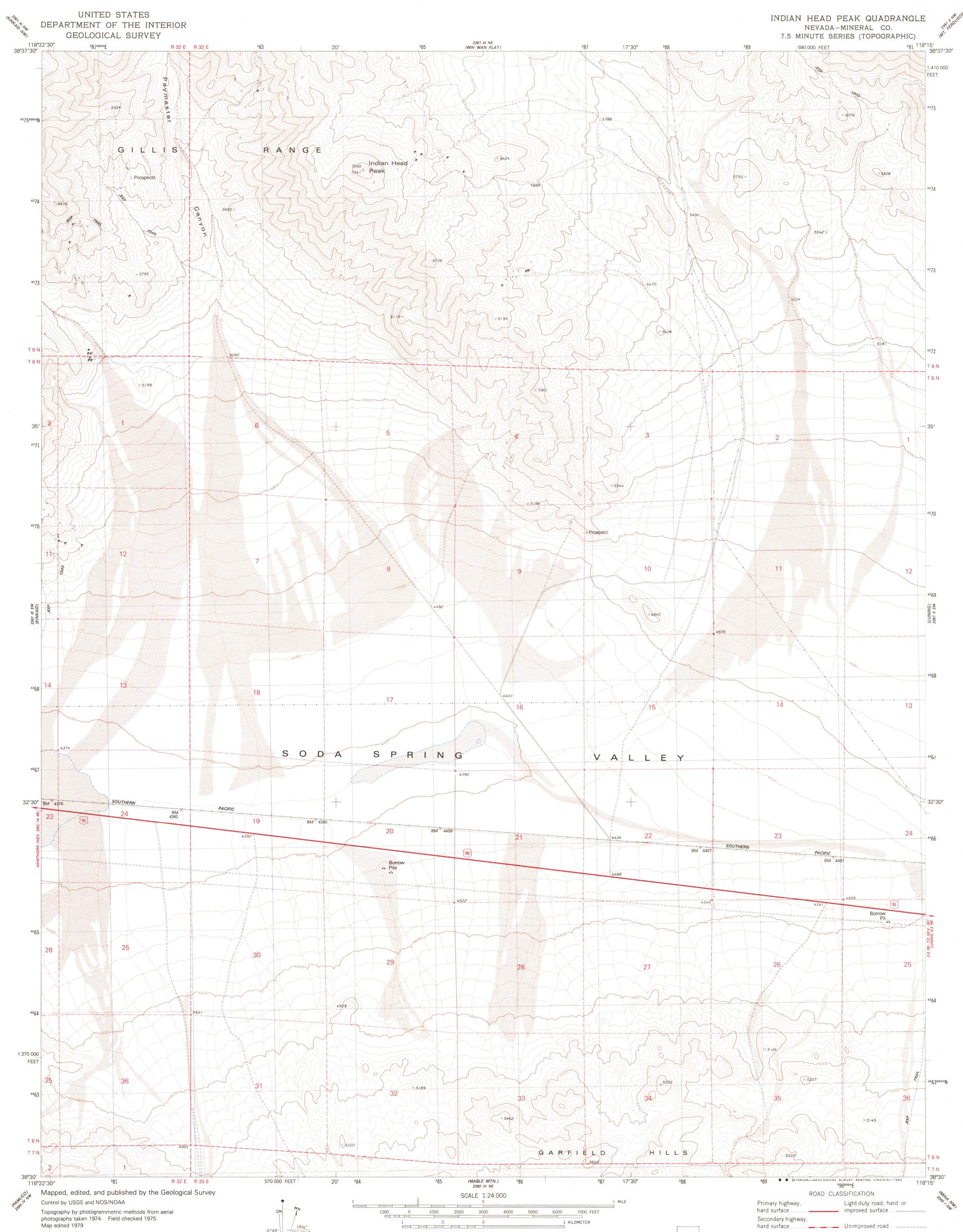
Projection and 10,000-foot grid ticks: Nevada coordinate system, west zone (transverse Mercator) 1000-meter Universal Transverse Mercator grid, zone 11 1927 North American Datum To place on the predicted North American Datum 1983 move the projection lines 12 meters north and 83 meters east as shown by dashed corner ticks Certain land lines are omitted, because of insufficient data
