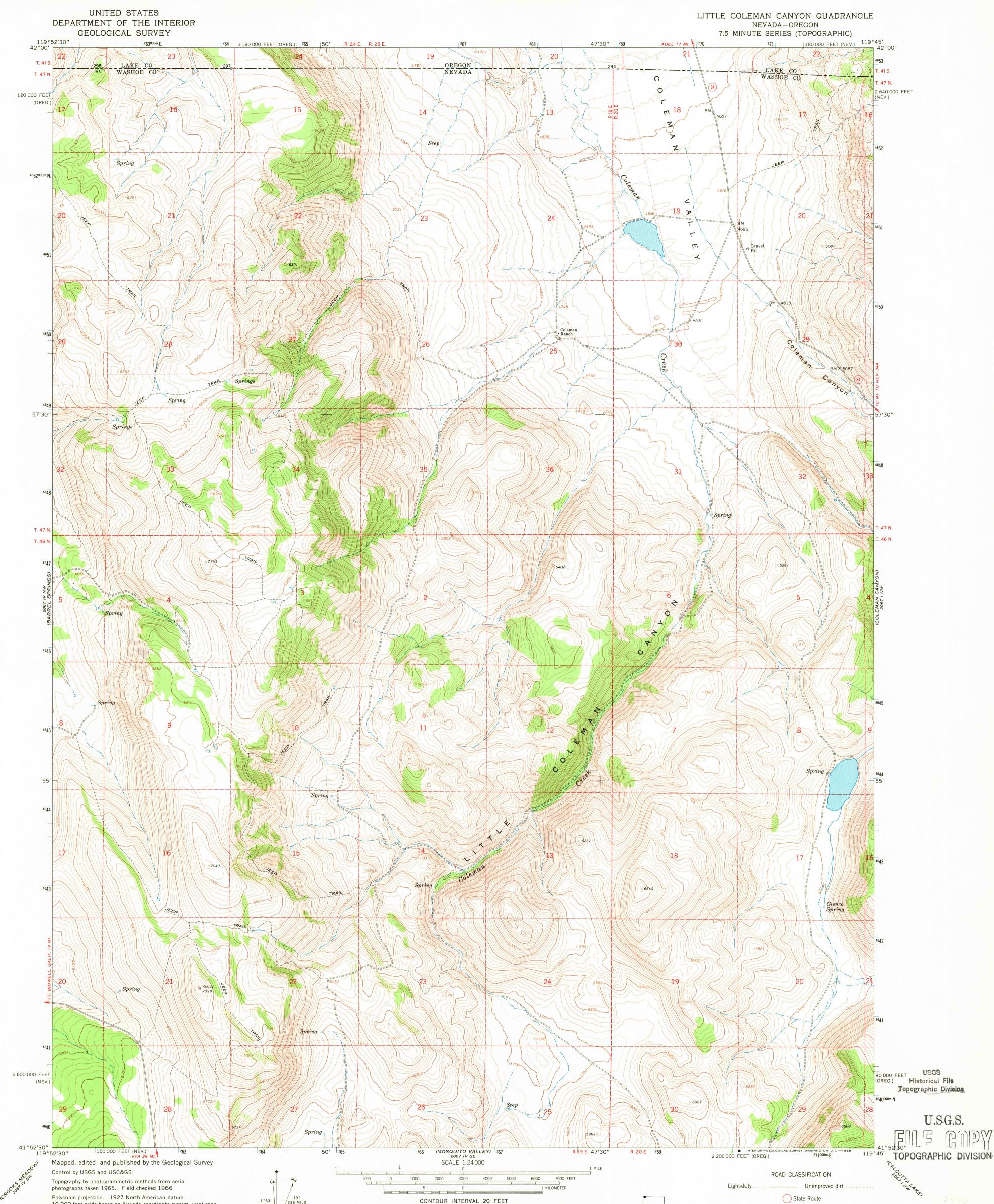
Polyconic projection. 1927 North American datum 10,000-foot grids based on Nevada coordinate system, west zone, and Oregon coordinate system, south zone 1000-meter Universal Transverse Mercator grid ticks, zone 11, shown in blue
