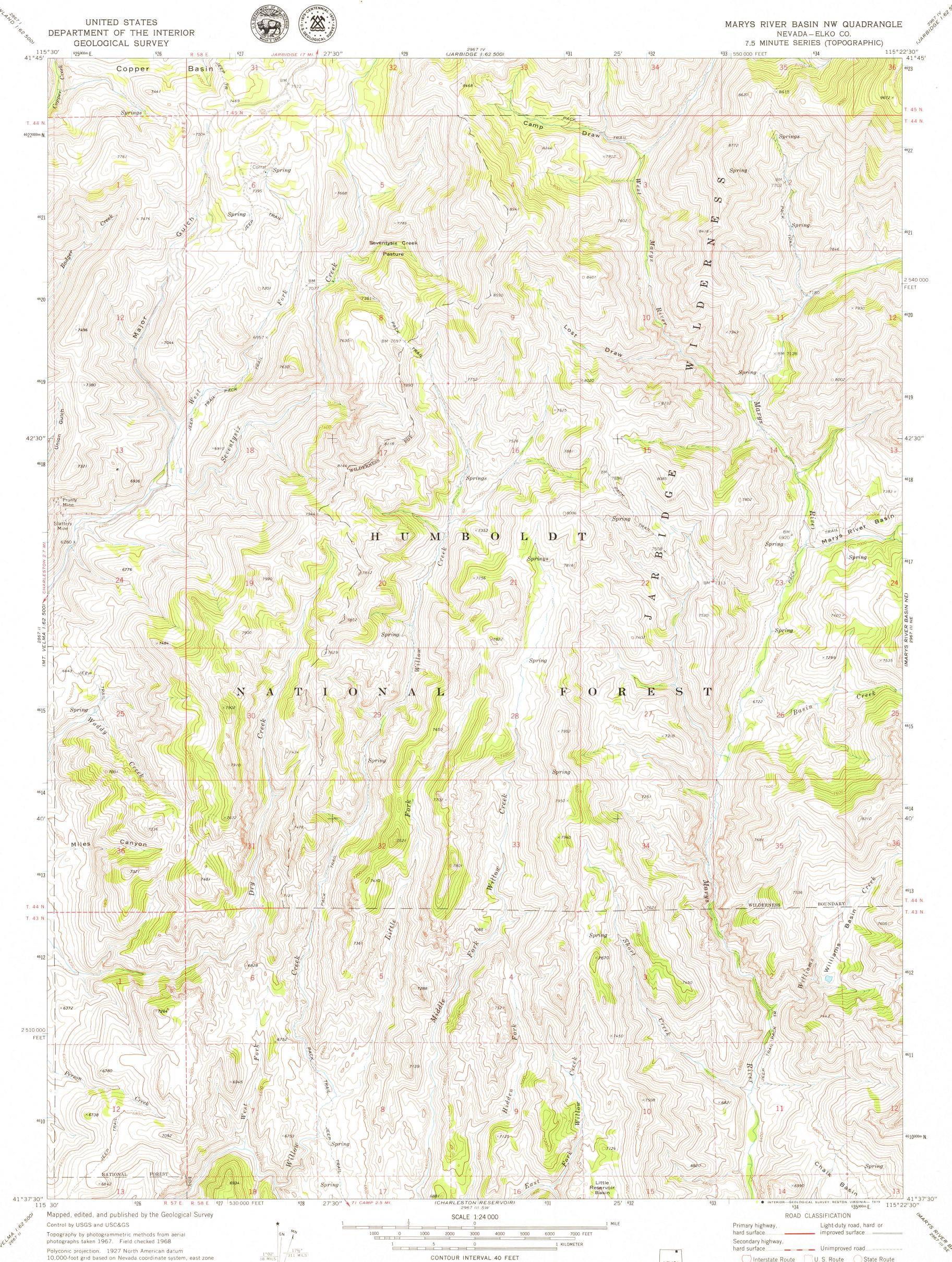
10,000-foot grid based on Nevada coordinate system, east zone 1000-meter Universal Transverse Mercator grid ticks, zone 11, shown in blue Fine red dashed lines indicate selected fence lines
