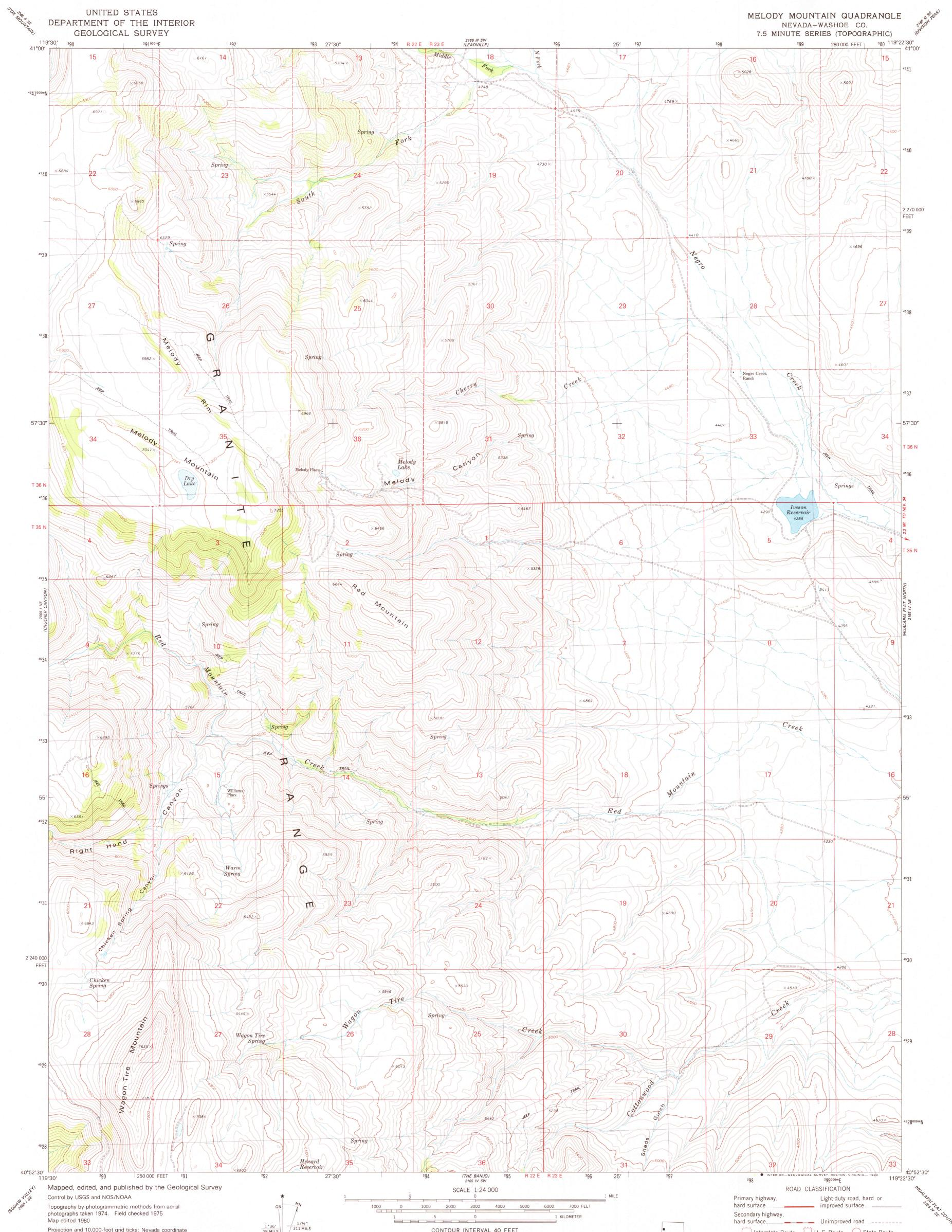
Projection and 10,000-foot grid ticks: Nevada coordinate system, west zone (transverse Mercator) 1000-meter Universal Transverse Mercator grid, zone 11 1927 North American Datum To place on the predicted North American Datum 1983 move the projection lines 16 meters north and 85 meters east as shown by dashed corner ticks Fine red dashed lines indicate selected fence and field lines where generally visible on aerial photographs. This information is unchecked
