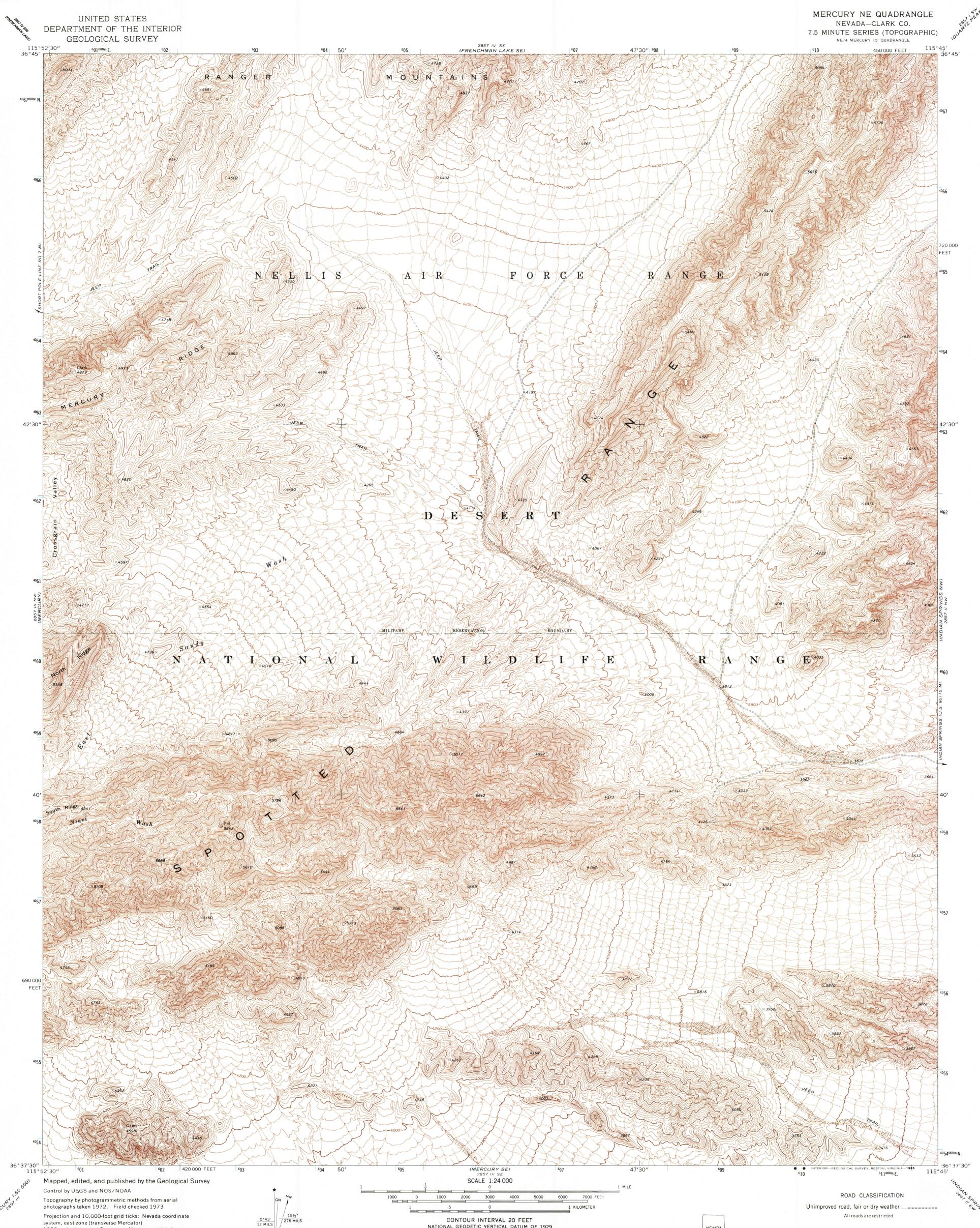
system, east zone (transverse Mercator) 1000-meter Universal Transverse Mercator grid ticks, zone 11, shown in blue. 1927 North American datum To place on the predicted North American Datum 1983 move the projection lines 7 meters porth and 77 meters east as shown by dashed corner ticks
