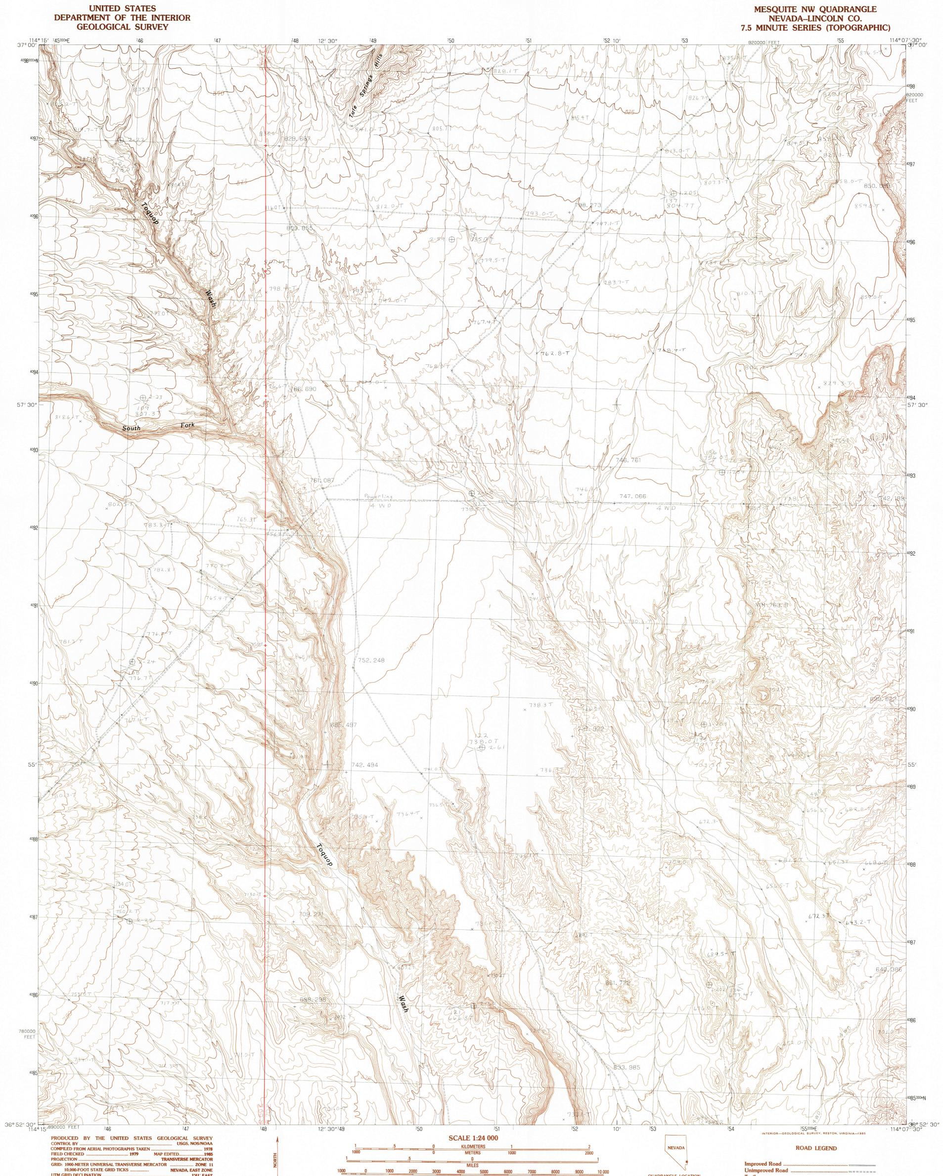
UTM GRID DECLINATION 1'41' EAST 1985 MAGNETIC NORTH DECLINATION 14° EAST VERTICAL DATUM NATIONAL GEODETIC VERTICAL DATUM OF 1929 HORIZONTAL DATUM 1927 NORTH AMERICAN DATUM To place on the predicted North American Datum of 1983, move the projection lines as shown by dashed corner ticks (6 meters north and 72 meters east) There may be private inholdings within the boundaries of any Federal and State Reservations shown on this map Where omitted, land lines have not been established
