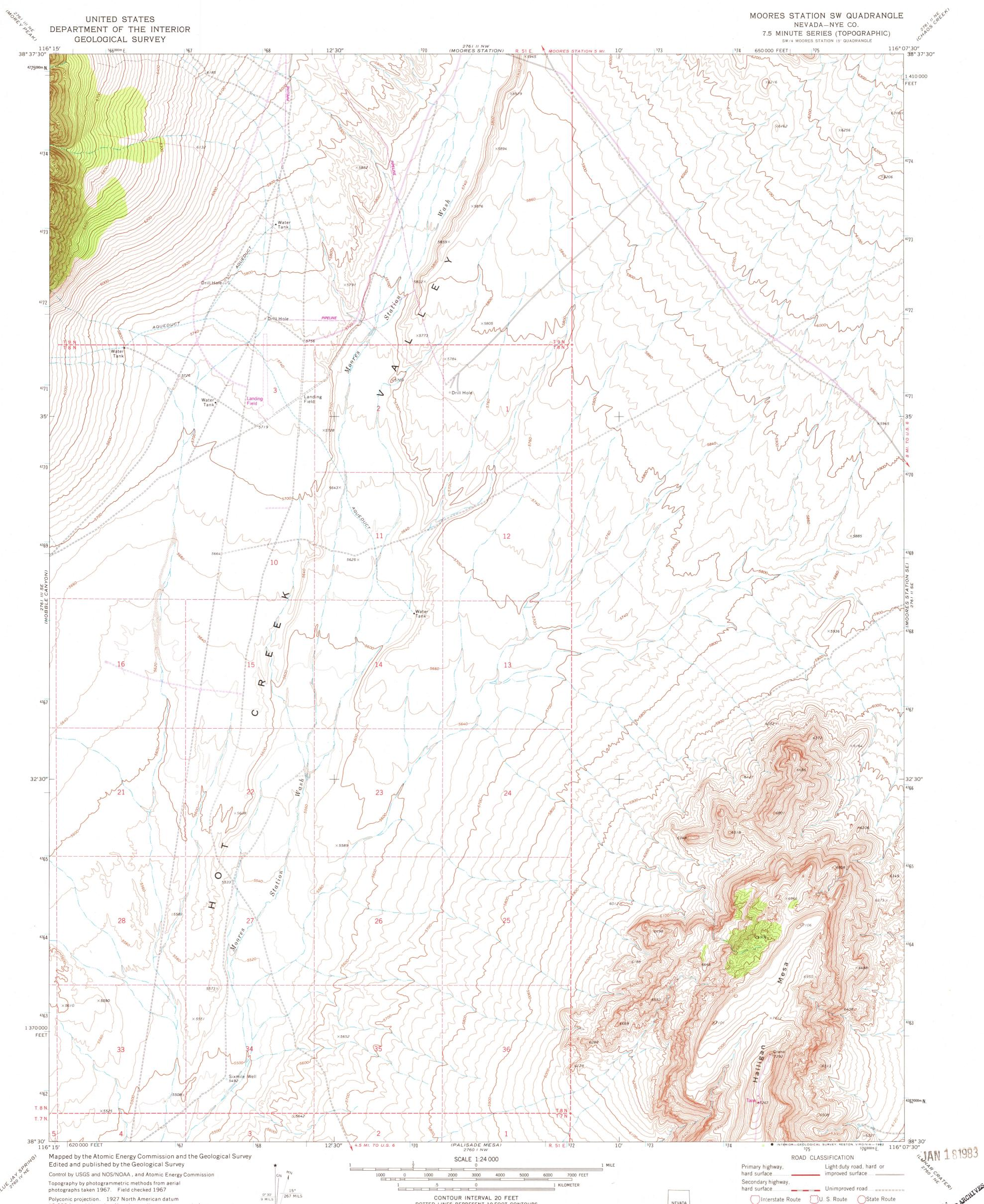
Polyconic projection. 1927 North American datum 10,000-foot grid based on Nevada coordinate system, central zone 1000-meter Universal Transverse Mercator grid ticks, zone 11, shown in blue To place on the predicted North American Datum 1983, move the projection lines 10 meters north and 77 meters east as shown by dashed corner ticks
