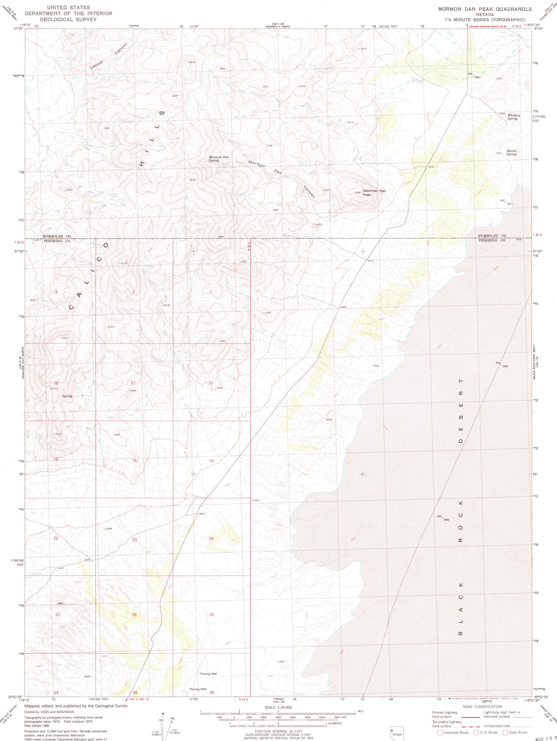
Projection and 10,000-foot grid ticks: Nevada coordinate system, west zone (transverse Mercator) 1000-meter Universal Transverse Mercator grid, zone 11 1927 North American Datum To place on the predicted North American Datum 1983 move the projection lines 15 meters north and 85 meters east as shown by dashed corner ticks Fine red dashed lines indicate selected fence and field lines where generally visible on aerial photographs. This information is unchecked
