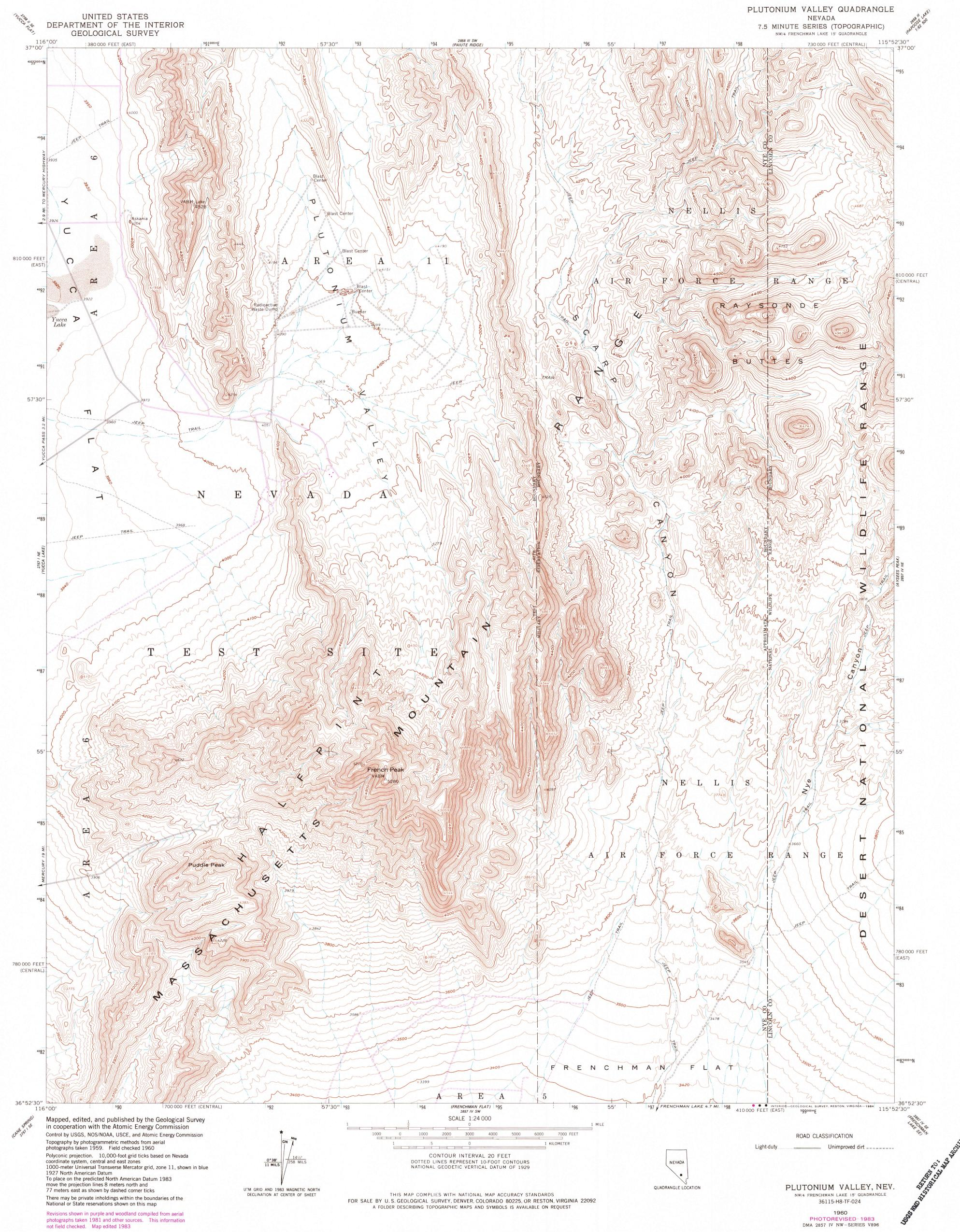
Polyconic projection. 10,000-foot grid ticks based on Nevada coordinate system, central and east zones 1000-meter Universal Transverse Mercator grid, zone 11, shown in blue 1927 North American Datum To place on the predicted North American Datum 1983 move the projection lines 8 meters north and 77 meters east as shown by dashed corner ticks
