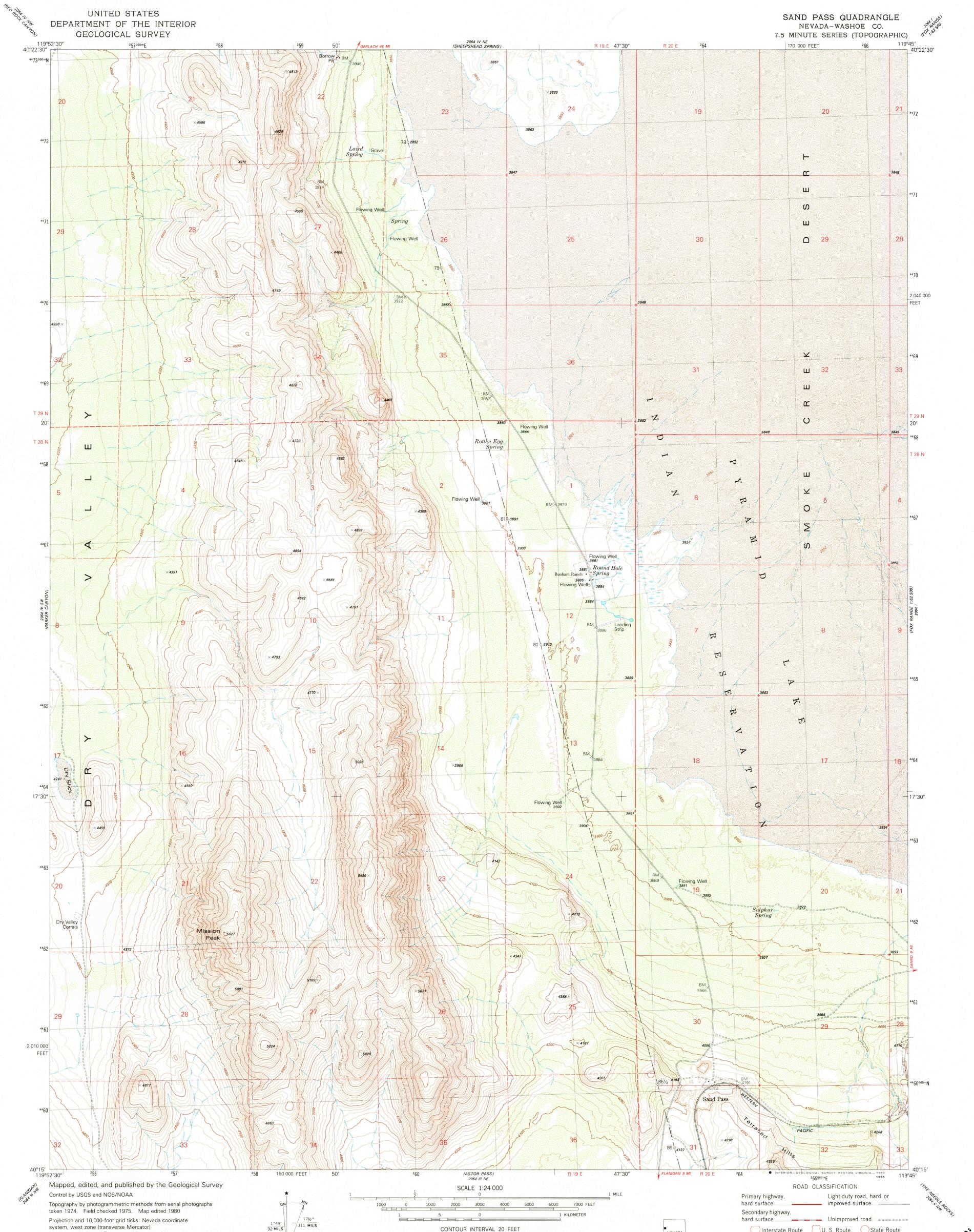
Projection and 10,000-foot grid ticks: Nevada coordinate system, west zone (transverse Mercator) 1000-meter Universal Transverse Mercator grid, zone 11 1927 North American Datum To place on the predicted North American Datum 1983 move the projection lines 15 meters north and 87 meters east as shown by dashed corner ticks
