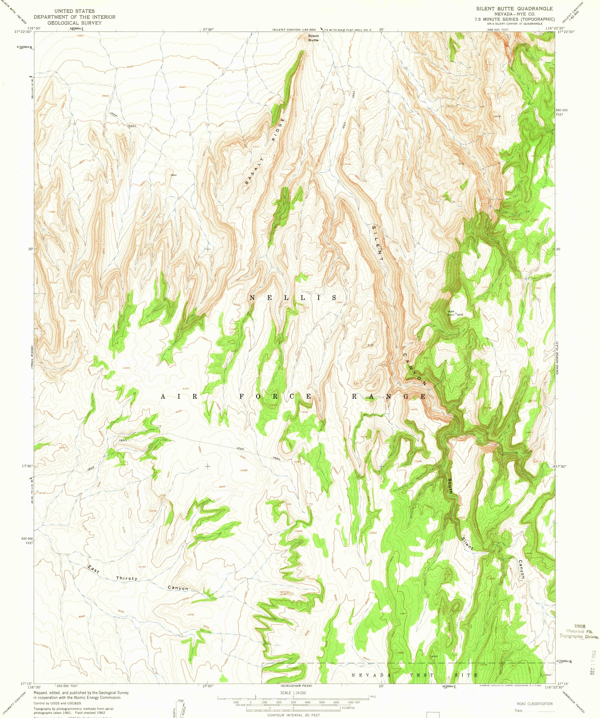
Polyconic projection. 1927 North American datum 10,000-foot grid based on Nevada coordinate system, central zone 1000-meter Universal Transverse Mercator grid ticks, zone 11, shown in blue
