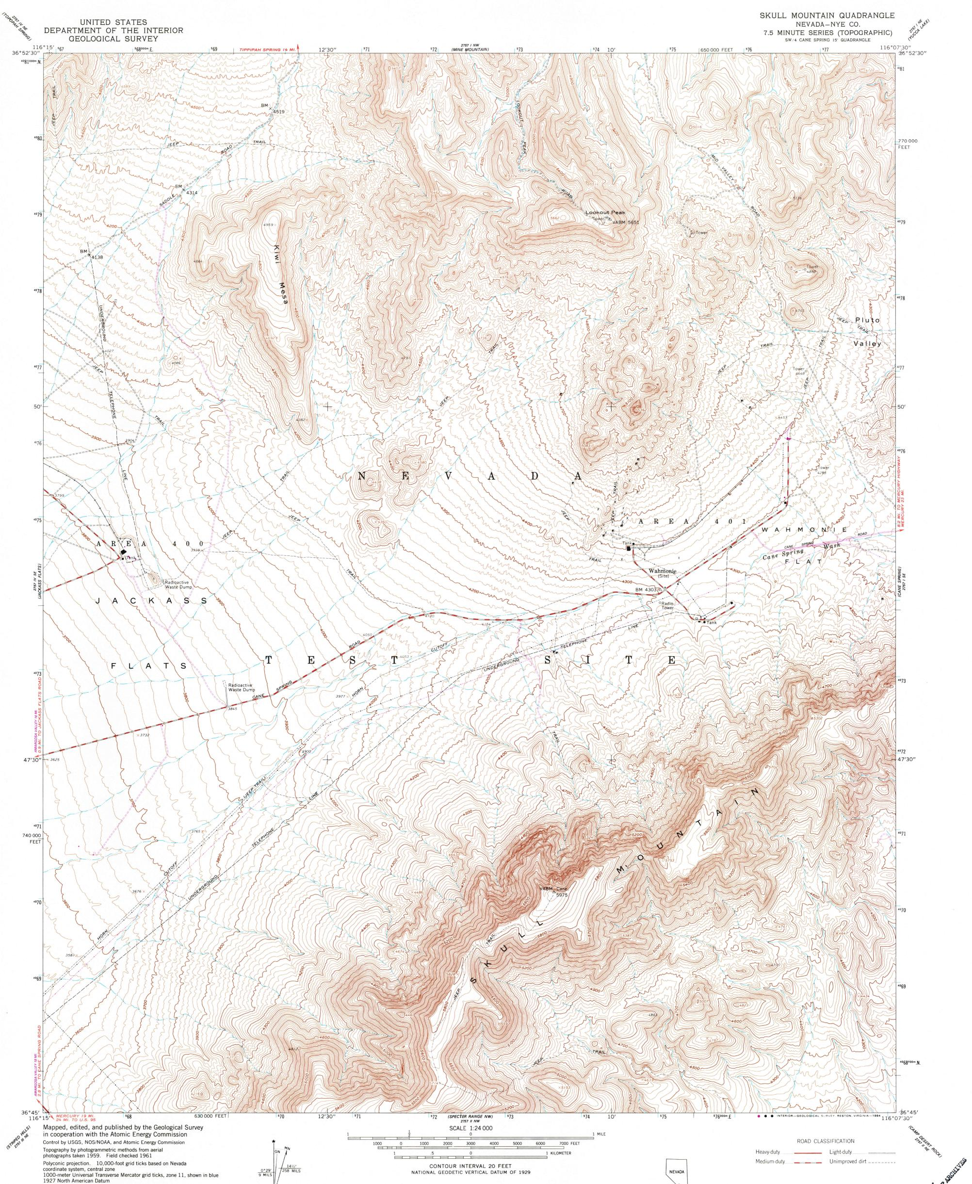
Polyconic projection. 10,000-foot grid ticks based on Nevada coordinate system, central zone 1000-meter Universal Transverse Mercator grid ticks, zone 11, shown in blue 1927 North American Datum To place on the predicted North American Datum 1983 move the projection lines 8 meters north and 78 meters east as shown by dashed corner ticks
