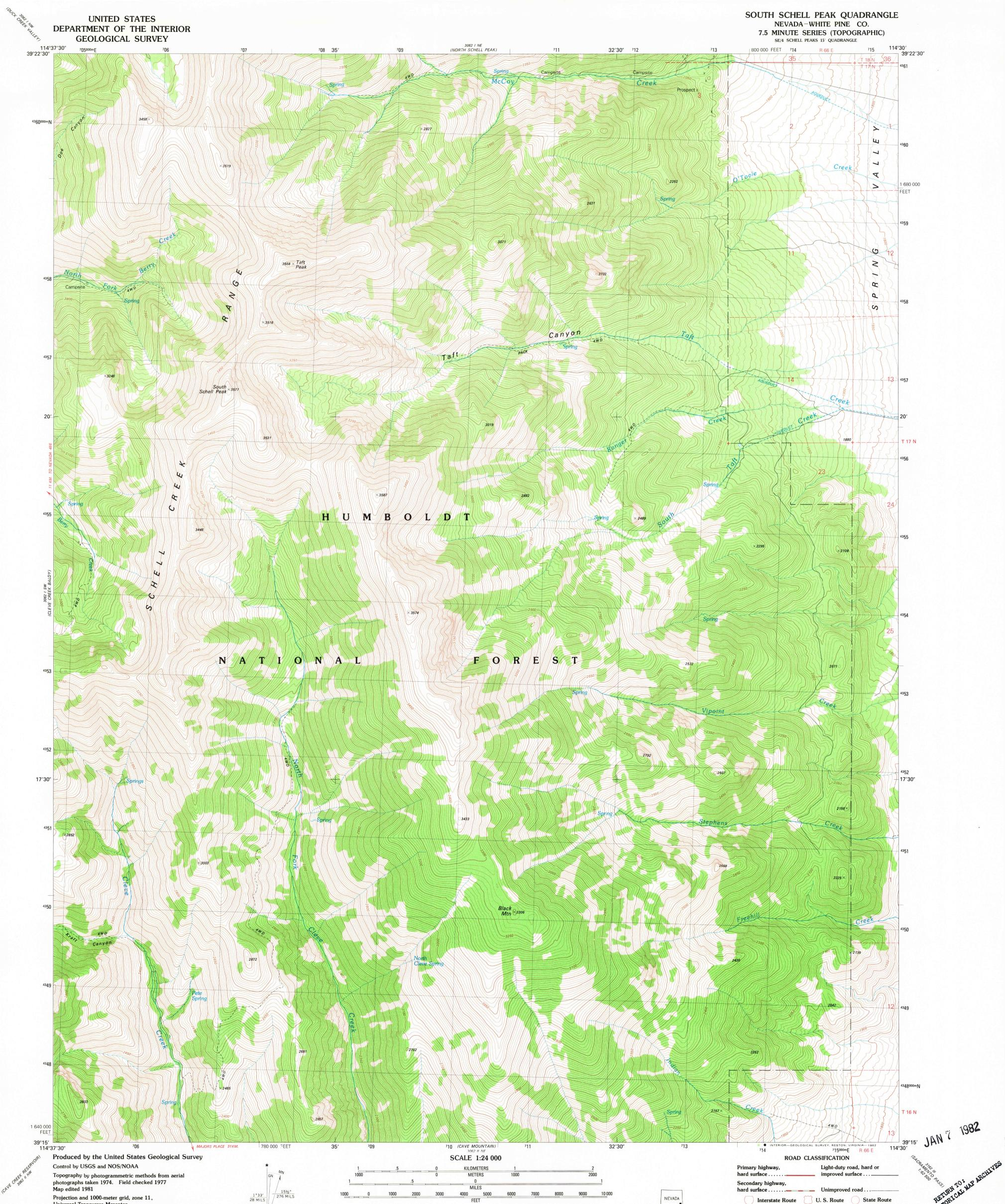
Projection and 1000-meter grid, zone 11, Universal Transverse Mercator 10,000-foot grid ticks based on Nevada coordinate system, east zone. 1927 North American Datum To place on the predicted North American Datum 1983 move the projection lines 10 meters north and 73 meters east as shown by dashed corner ticks Where omitted, land lines have not been established There may be private inholdings within the boundaries of the National or State reservations shown on this map
