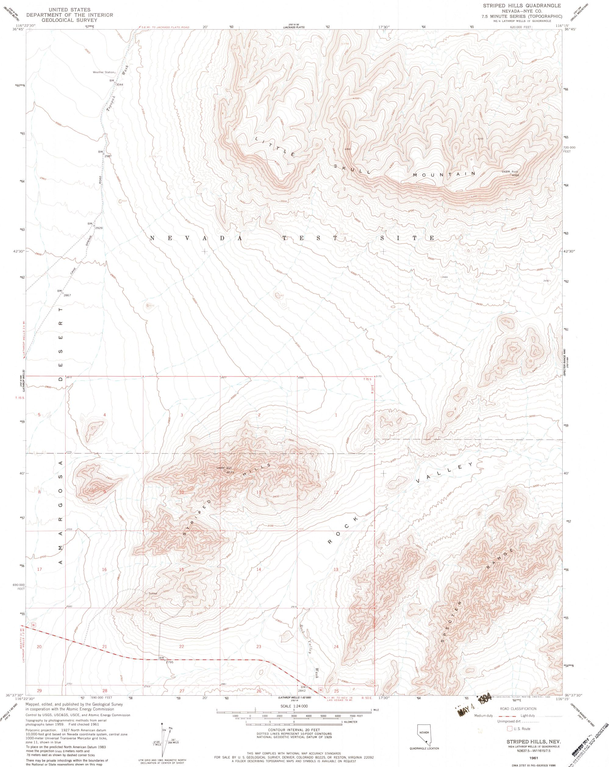
Polyconic projection. 1927 North American datum 10,000-foot grid based on Nevada coordinate system, central zone 1000-meter Universal Transverse Mercator grid ticks, zone 11, shown in blue To place on the predicted North American Datum 1983 move the projection lines 8 meters north and 78 meters east as shown by dashed corner ticks There may be private inholdings within the boundaries of the National or State reservations shown on this map
