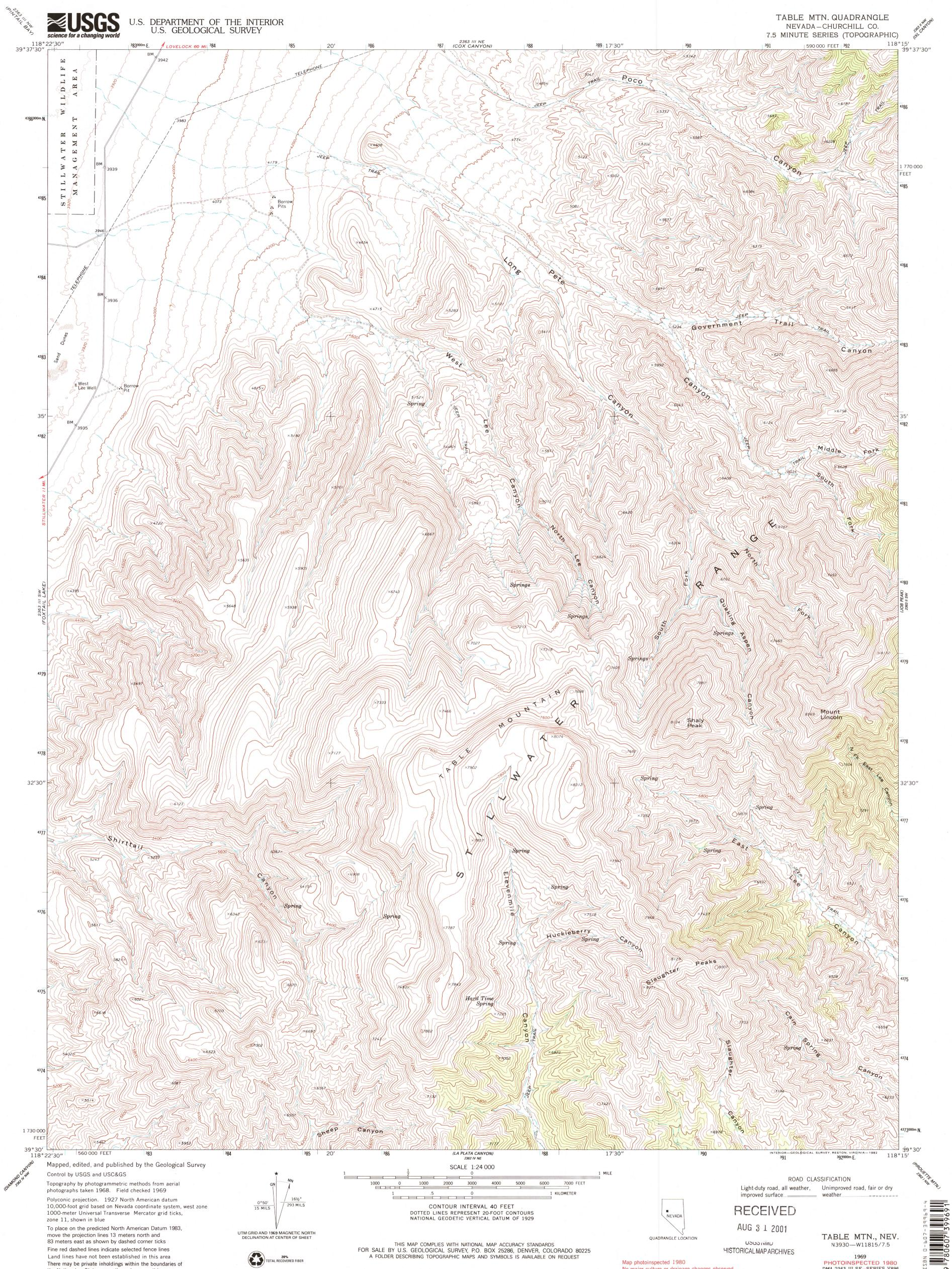
10,000-foot grid based on Nevada coordinate system, west zone 1000-meter Universal Transverse Mercator grid ticks, zone 11, shown in blue To place on the predicted North American Datum 1983, move the projection lines 13 meters north and 83 meters east as shown by dashed corner ticks Fine red dashed lines indicate selected fence lines Land lines have not been established in this area There may be private inholdings within the boundaries of the National or State reservations shown on this map
