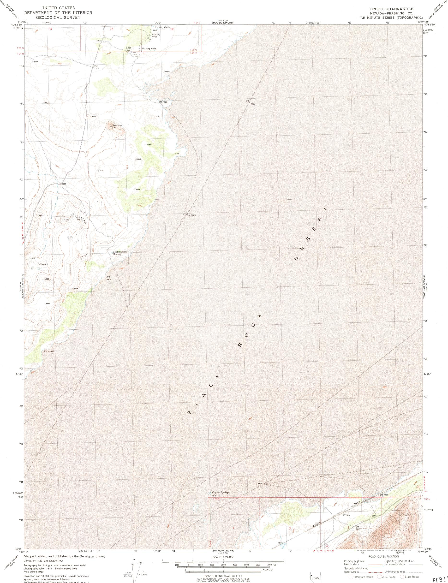
Projection and 10,000-foot grid ticks: Nevada coordinate system, west zone (transverse Mercator) 1000-meter Universal Transverse Mercator grid, zone 11 1927 North American Datum To place on the predicted North American Datum 1983 move the projection lines 15 meters north and 85 meters east as shown by dashed corner ticks Fine red dashed lines indicate selected fence and field lines where
