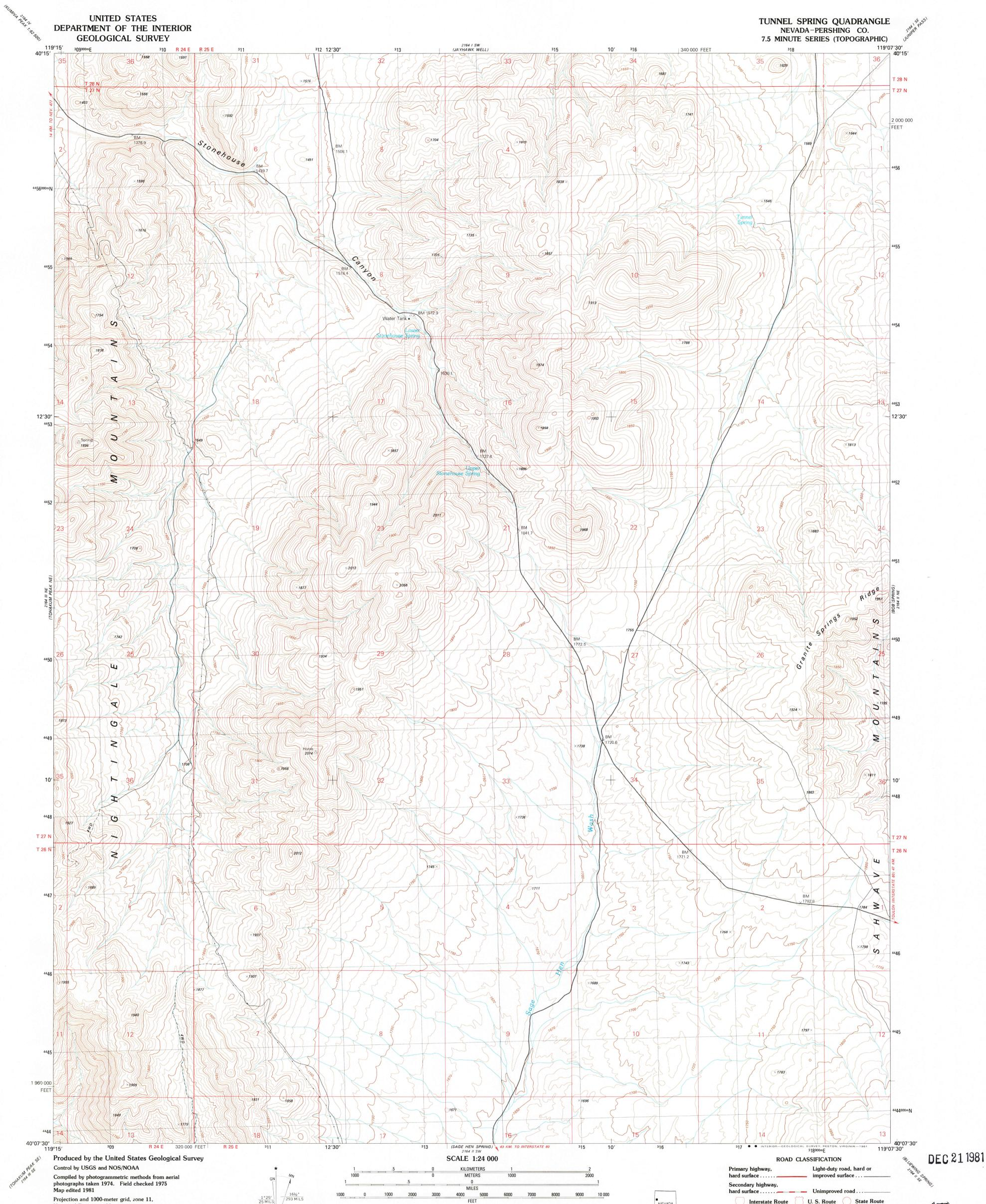
Projection and 1000-meter grid, zone 11, Universal Transverse Mercator 10,000-foot grid ticks based on Nevada coordinate system, west zone. 1927 North American Datum To place on the predicted North American Datum 1983 move the projection lines 14 meters north and 86 meters east as shown by dashed corner ticks
