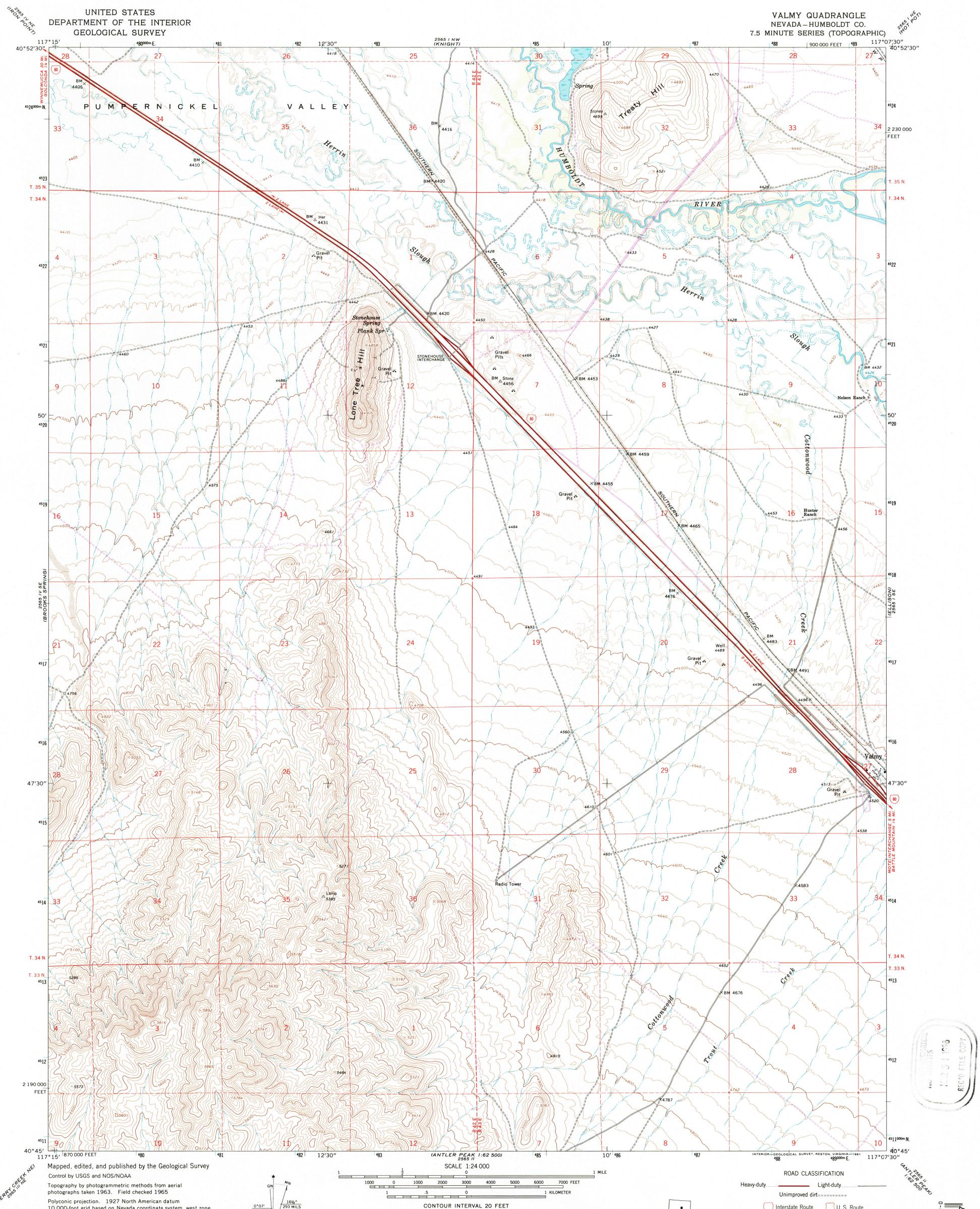
10,000-foot grid based on Nevada coordinate system, west zone 1000-meter Universal Transverse Mercator grid ticks, zone 11, shown in blue To place on the predicted North American Datum 1983 move the projection lines 14 meters north and 80 meters east as shown by dashed corner ticks
