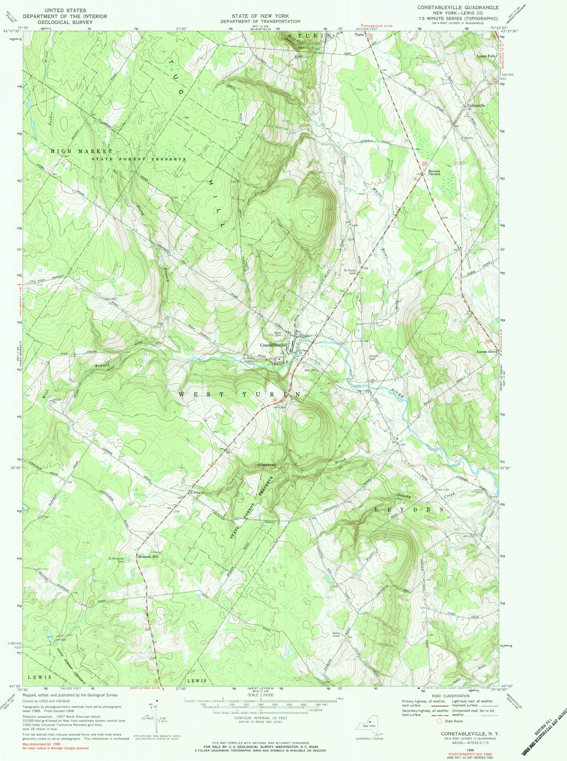
Polyconic projection. 1927 North American datum 10,000-foot grid based on New York coordinate system, central zone 1000-meter Universal Transverse Mercator grid ticks, zone 18, shown in blue
