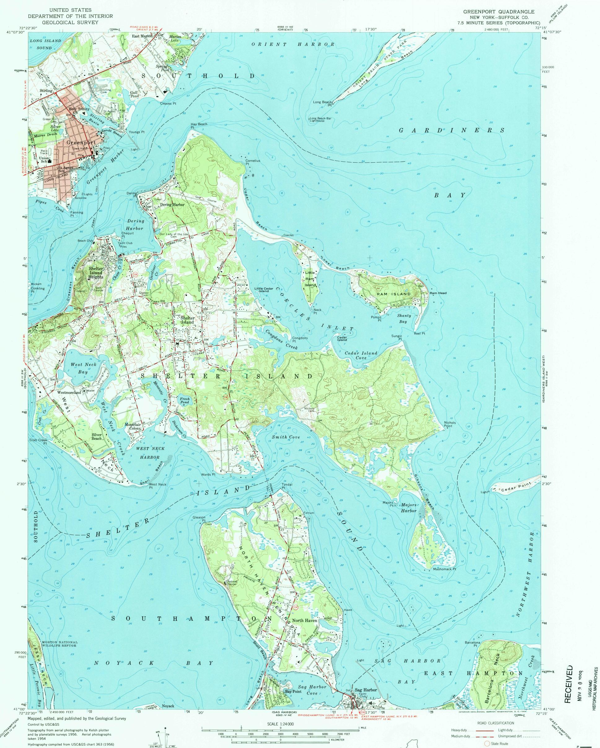
Hydrography compiled from USC&GS chart 363 (1956) Polyconic projection. 1927 North American datum 10,000-foot grid based on New York coordinate system, Long Island zone 1000-meter Universal Transverse Mercator grid ticks, zone 18, shòwn in blue
