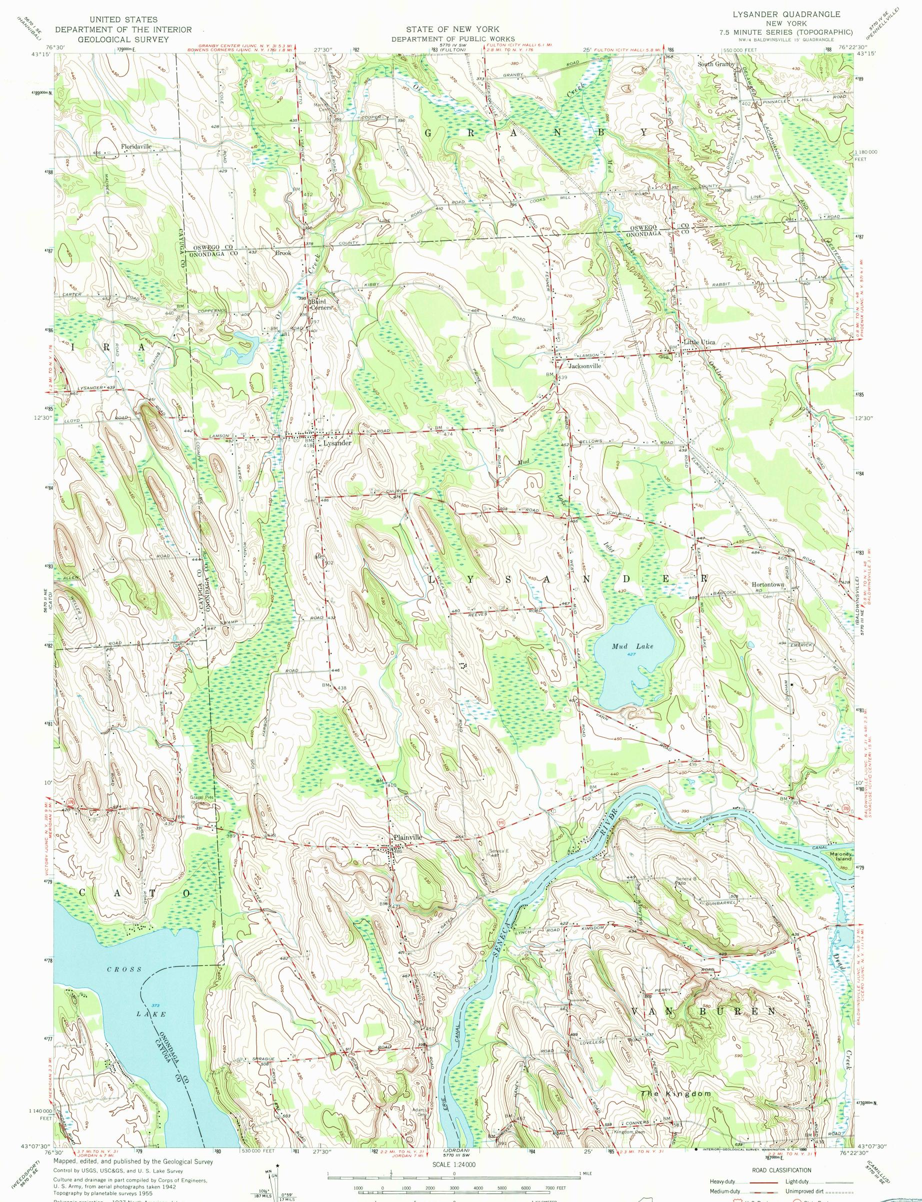
Polyconic projection. 1927 North American datum 10,000-foot grid based on New York coordinate system, central zone 1000-meter Universal Transverse Mercator grid ticks, zone 18, shown in blue
