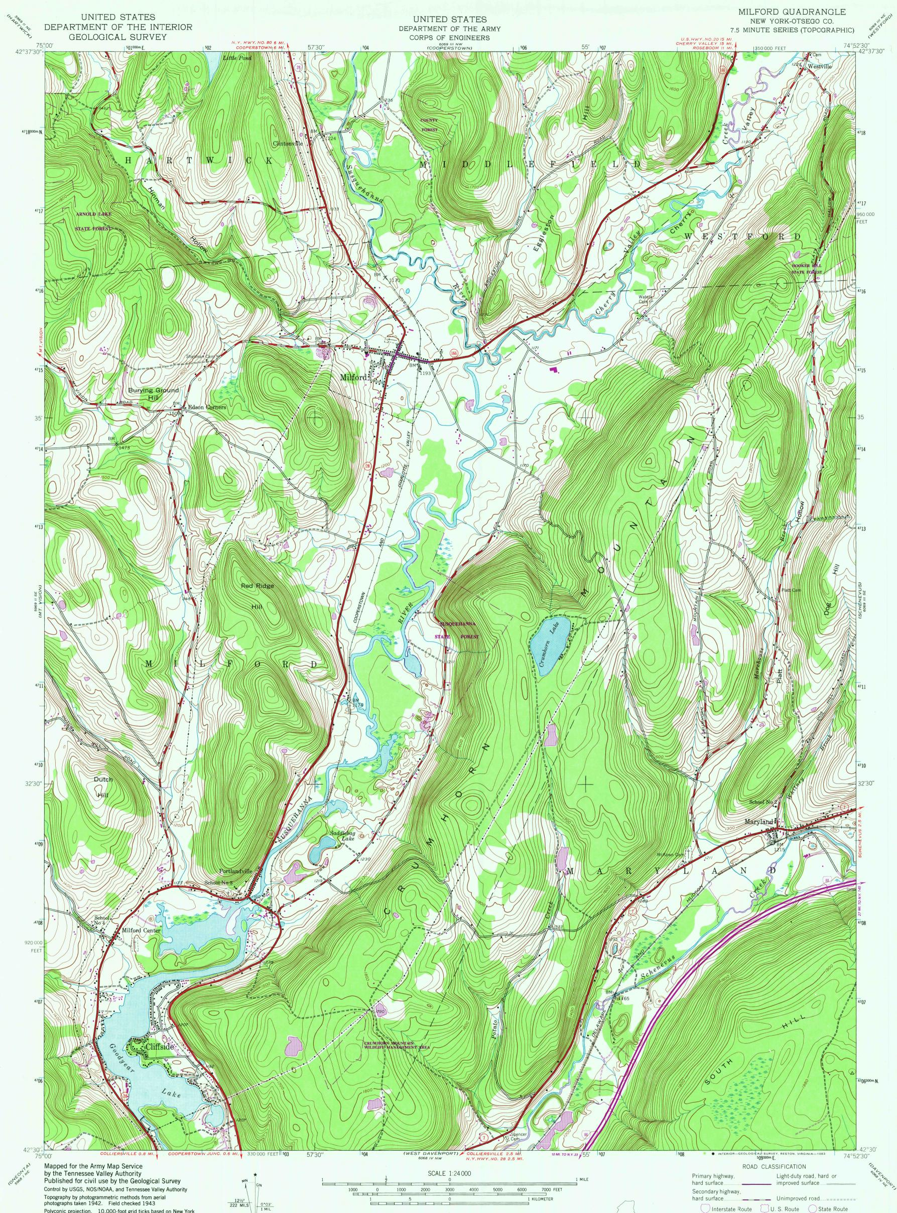
Topography by photogrammetric methods from aerial photographs taken 1942. Field checked 1943 Polyconic projection. 10,000-foot grid ticks based on New York coordinate system, east zone. 1000-meter Universal Transverse Mercator grid ticks, zone 18, shown in blue. 1927 North American Datum. To place on the predicted North American Datum 1983 move the projection lines 4 meters south and 31 meters west as shown by dashed corner ticks
